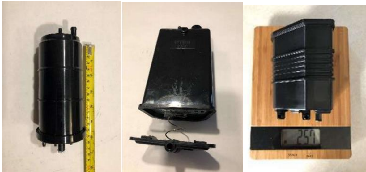
Figure 5: Different Shapes and Sizes of Carbon Canisters
