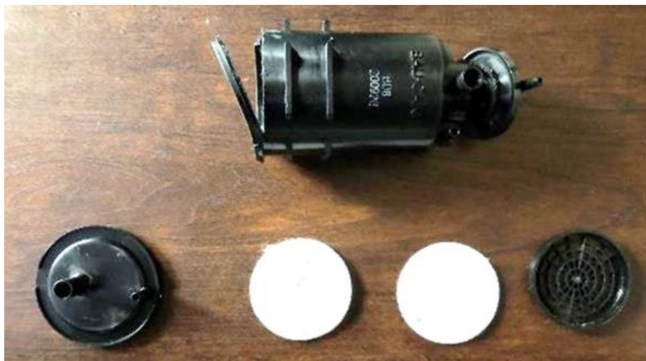
Figure 6: Carbon Canister Components
