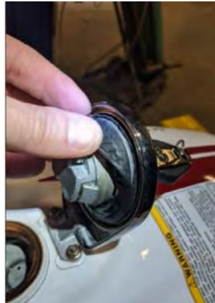
Figure 16: Degraded seal from leaking ONMC fuel cap
