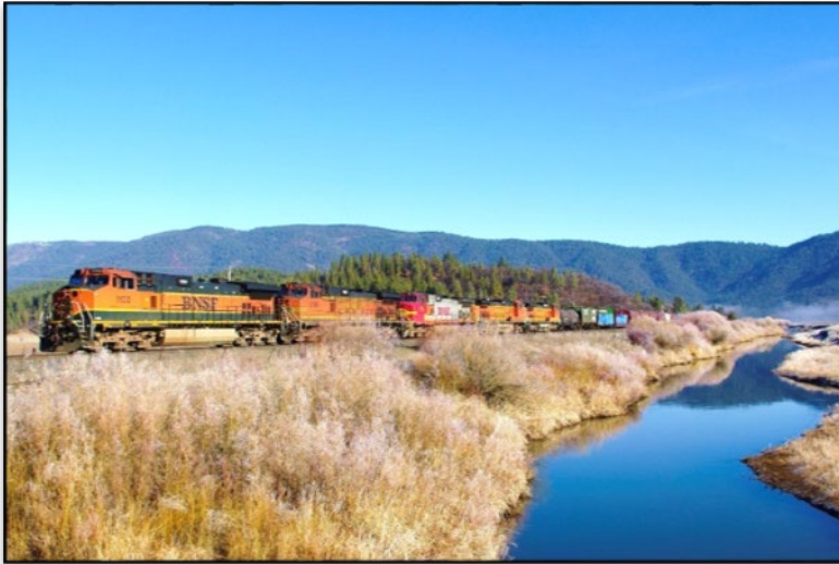
Figure 13: Class I line haul locomotives. Five line haul locomotives are working as a locomotive consist in this train
