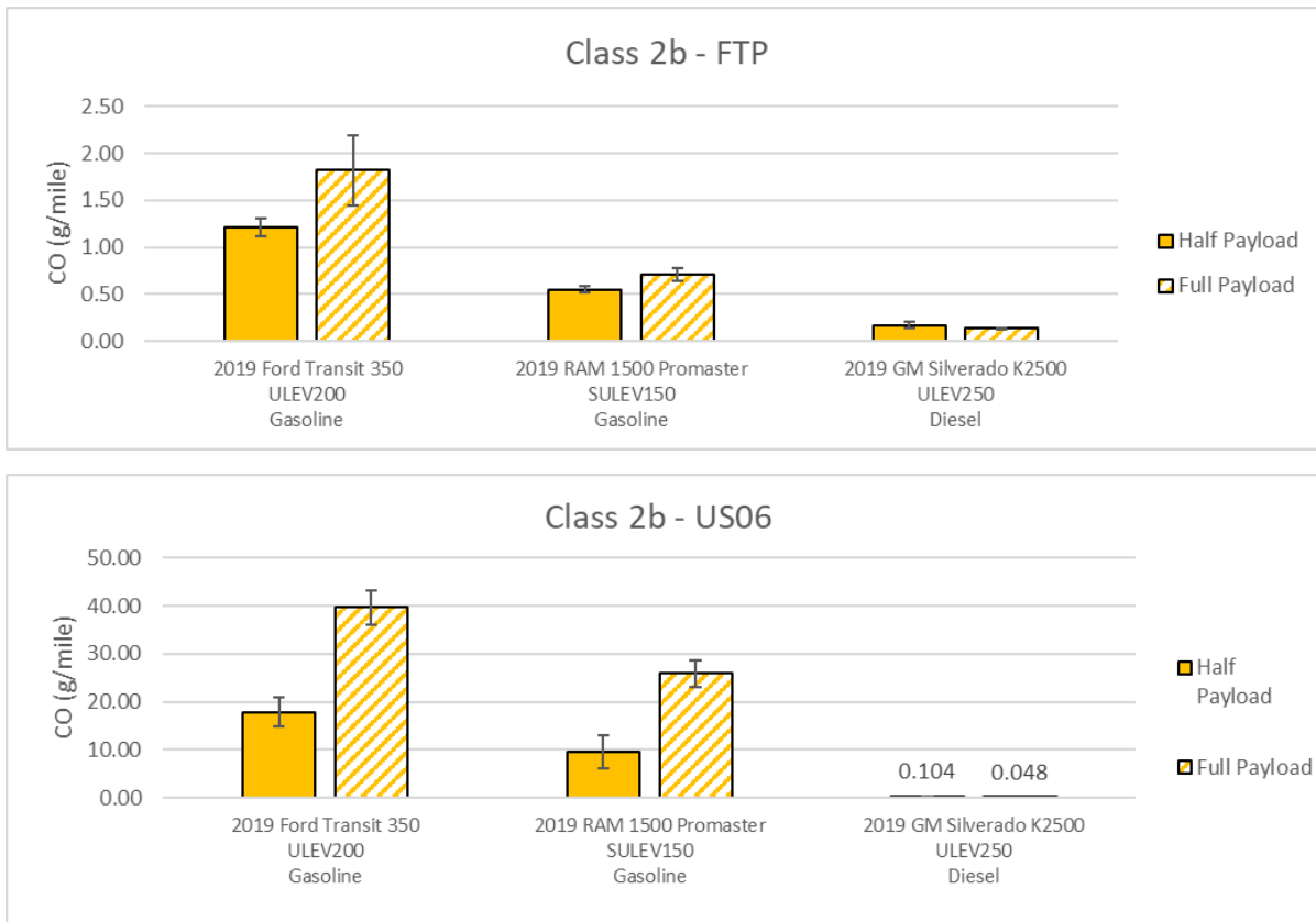
Figure 29: CARB’s MDV Test Data for CO at Half and Full Payload
