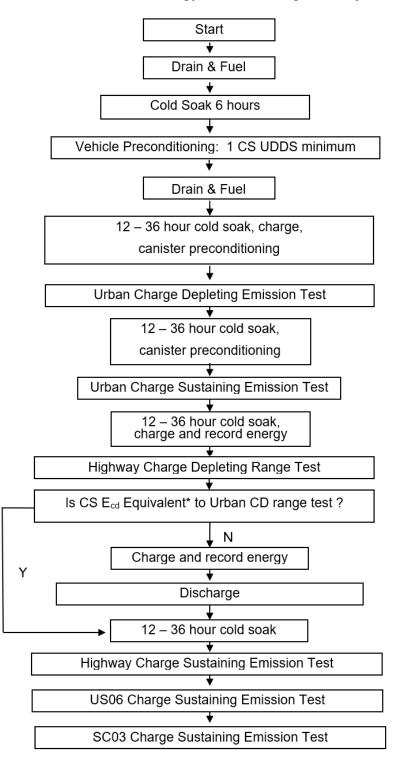
2. Example of an Off-Vehicle Charge Capable HEV with AER and Blended Operation Undergoing the Urban Charge Depleting Range Test.
