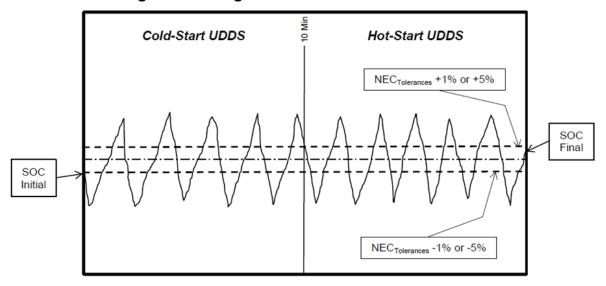
16. Urban Charge-Sustaining Emission Test – Valid Test.
