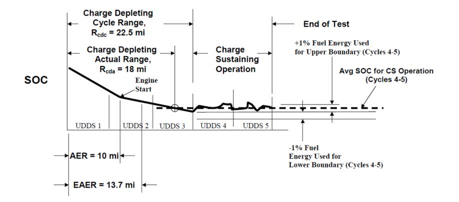
3. Example of Urban End of Test Conditions for a Plug-in Hybrid Electric Vehicle with and without Transitional Range.
