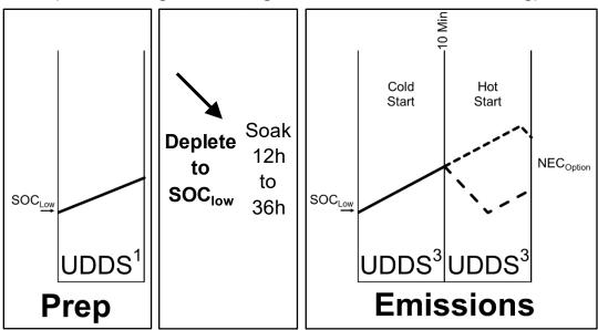
13. Urban Charge-Depleting Emission Test with Charge-Increasing Operation (not for charge-increasing driver-selectable mode testing).
