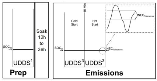
5. Urban Charge-Sustaining Emission Test with Charge-Increasing Driver-Selectable Mode Activated.
