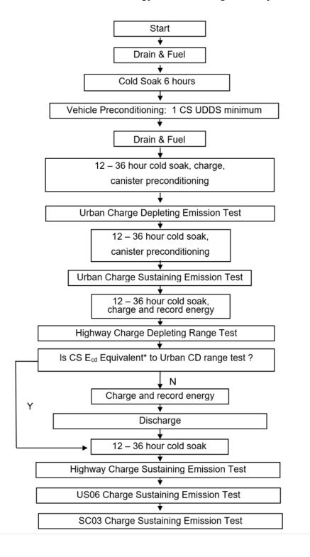
2. Example of an Off-Vehicle Charge Capable HEV with AER and Blended Operation Undergoing the Urban Charge Depleting Range Test.
