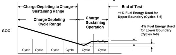
Example of Urban End of Test Conditions for a PHEV with Transitional Range
