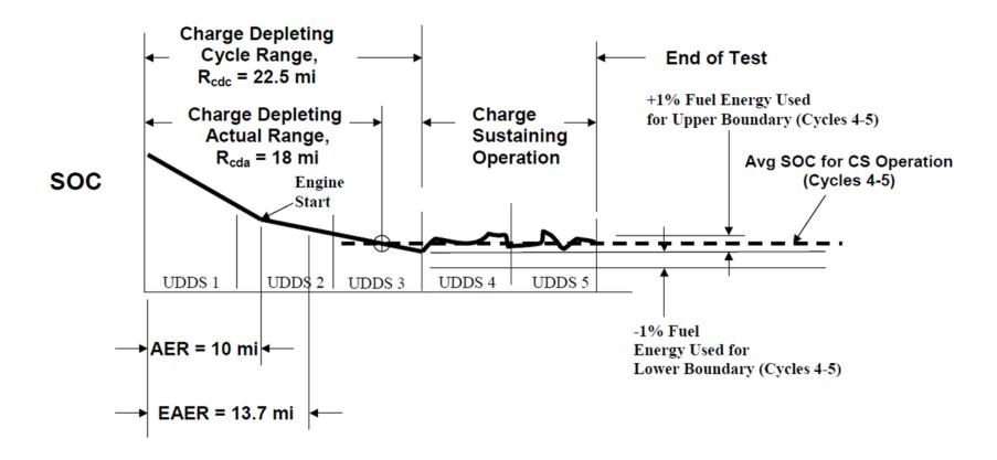
3. Example of Urban End of Test Conditions for a Plug-in Hybrid Electric Vehicle with and without Transitional Range.
