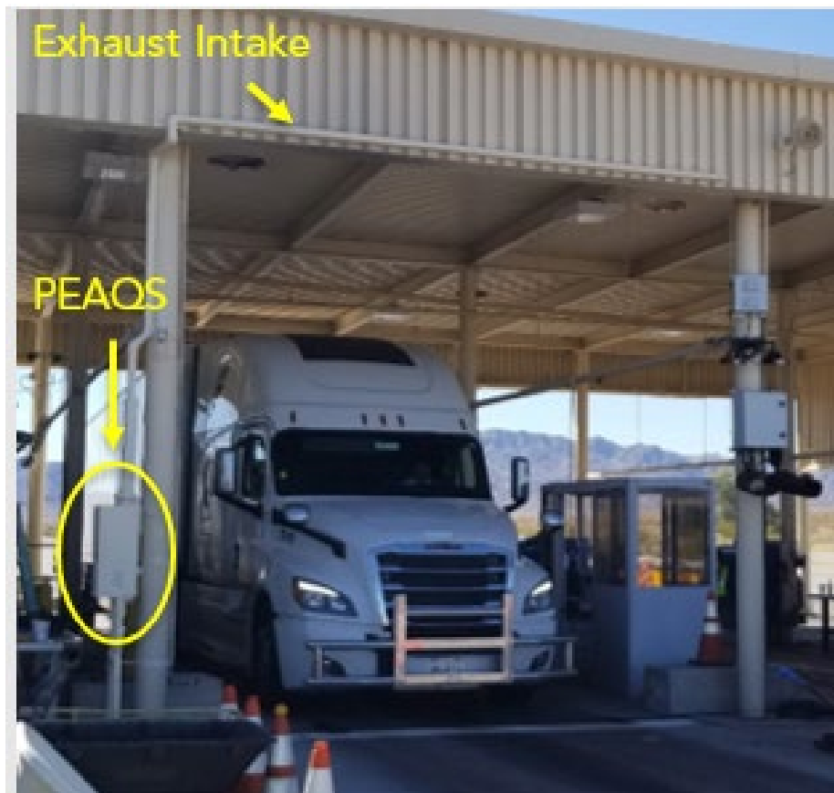
Figure III- 3: Example of Unattended PEAQS in Operation
