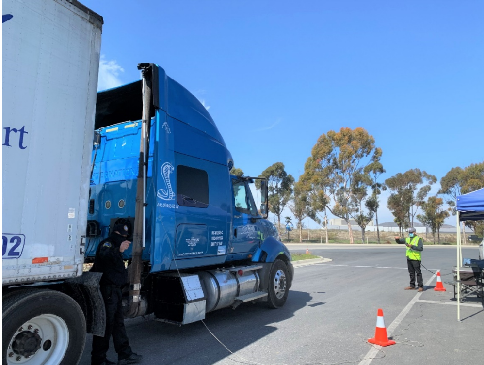
Figure III- 1: Smoke Opacity Test Performed at Vehicle Exhaust Tailpipe
