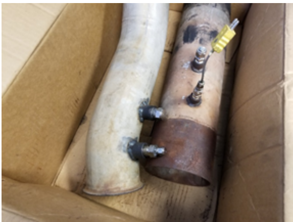
Figure 1. Sampling pores on exhaust elbow (left) for “engine out” exhaust emissions, and exhaust pipe for “tail-pipe” exhaust emissions (right)
