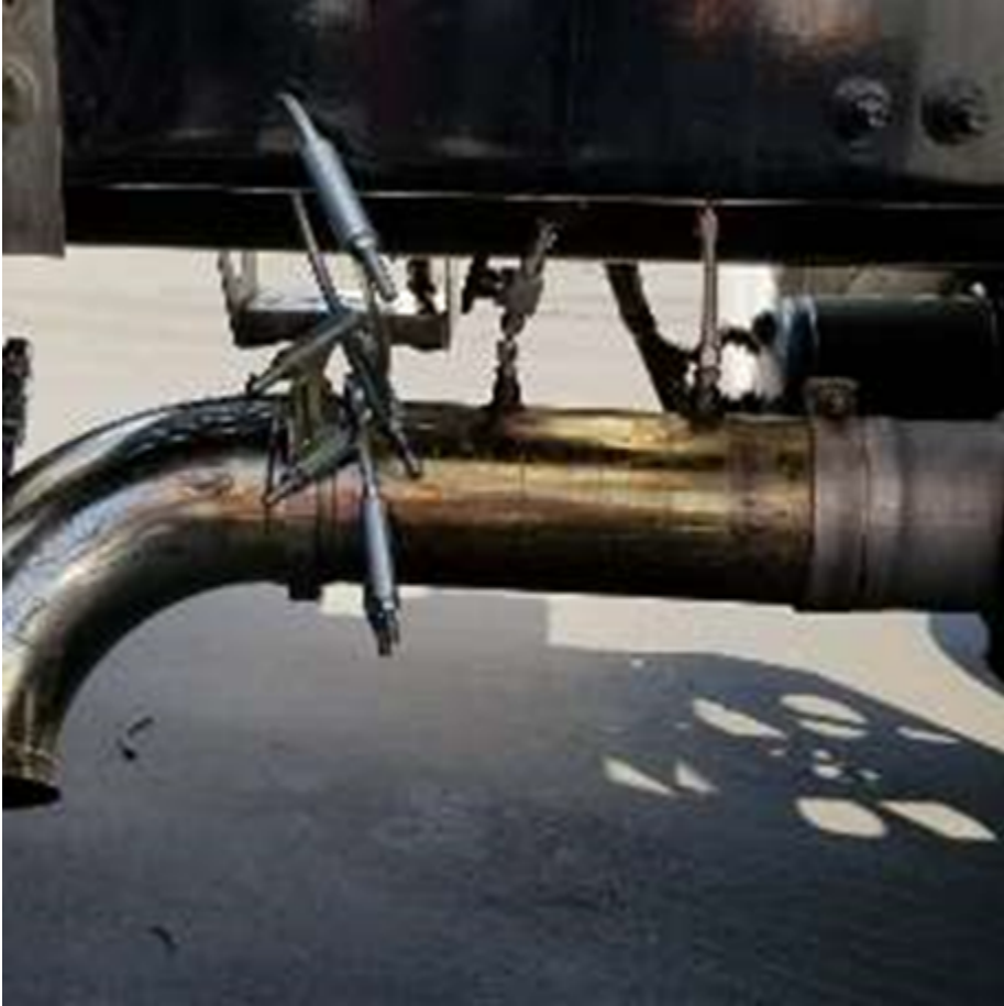
Figure 4. Exhaust pipe with sampling pores on a horizontal type exhaust
