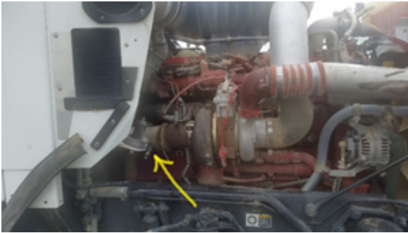
Figure 2. Exhaust elbow is located between the turbocharger outlet and one-box aftertreatment systems inlet.
