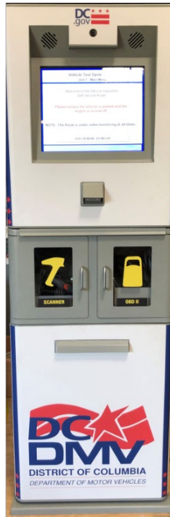
Figure 3-3 DC I/M Kiosk
