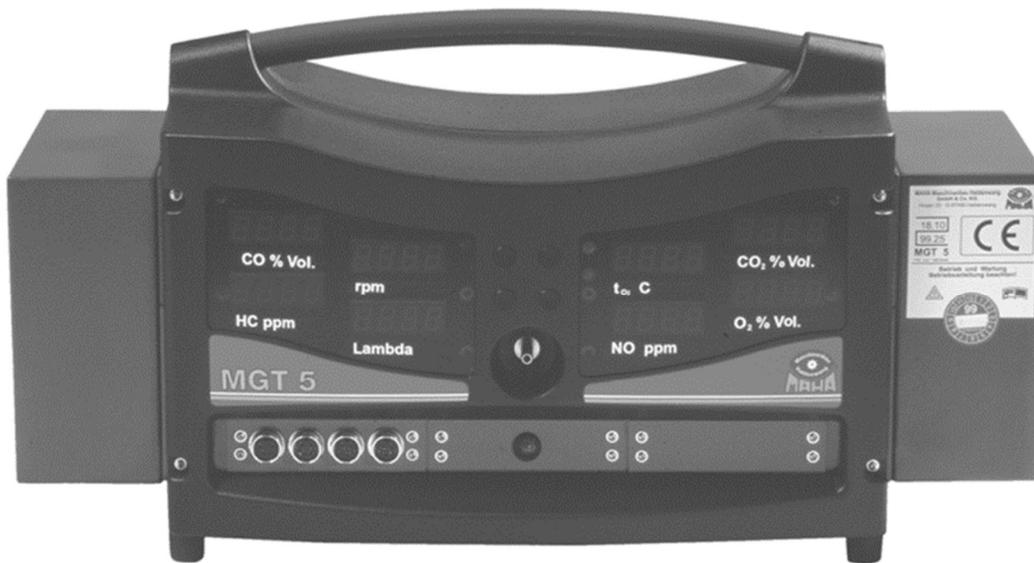
Figure C-1 Emissions Analyzers for Chassis Dynamometer Measurements
