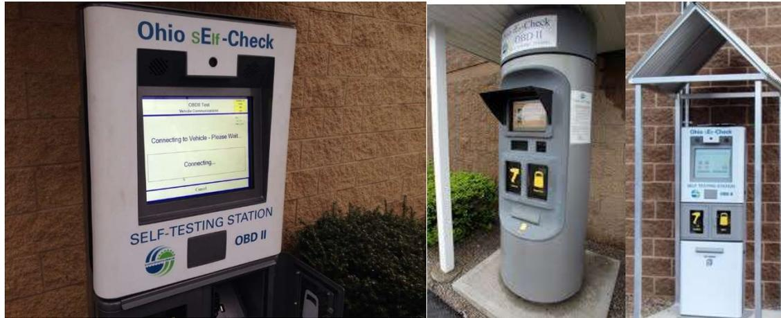
**Figure 2-11 Kiosk utilized for OBD scanning of LDVs**
