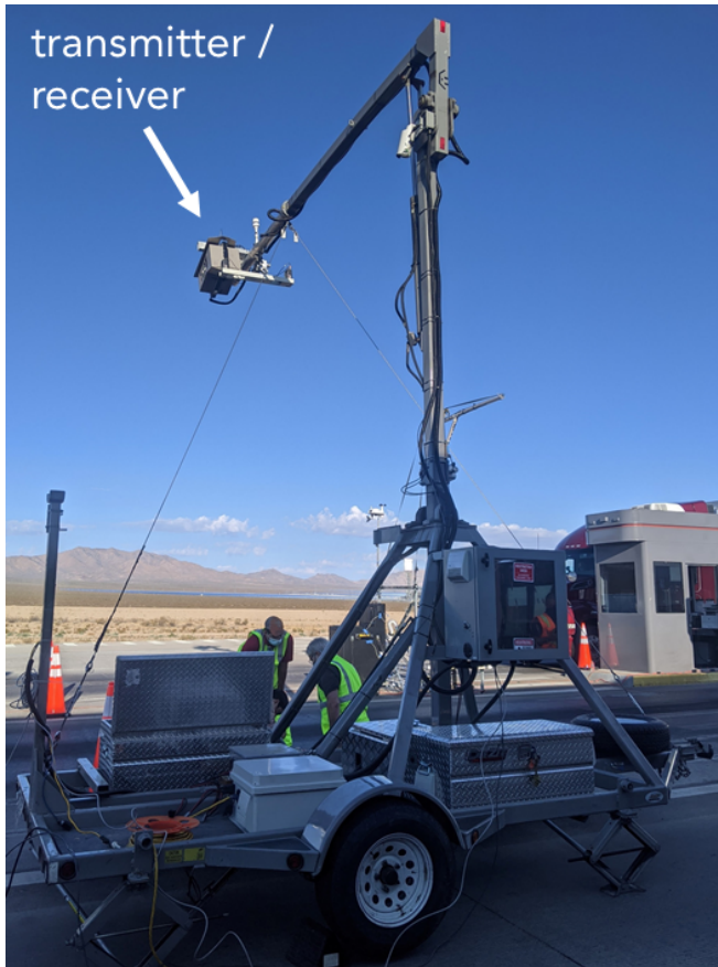
Figure 5-5. HEAT's EDAR system in operation at the Mt. Pass testing site. The combined transmitter/receiver is labelled.
