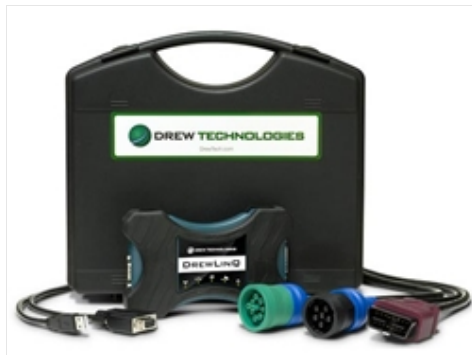
Figure 3-1. DrewLinQ OBD Data Collection Device.
