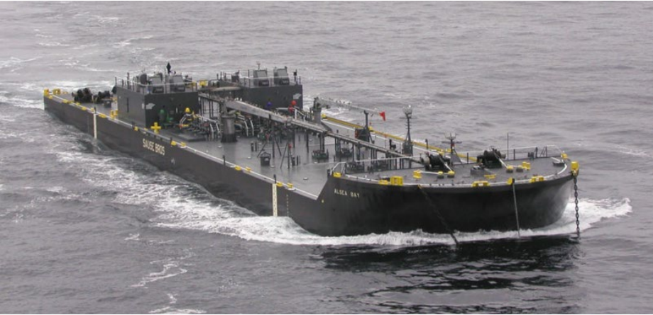
Figure A-3. Bernie Briere Double-Hull Fuel Bunker Barge at Port of San Francisco
