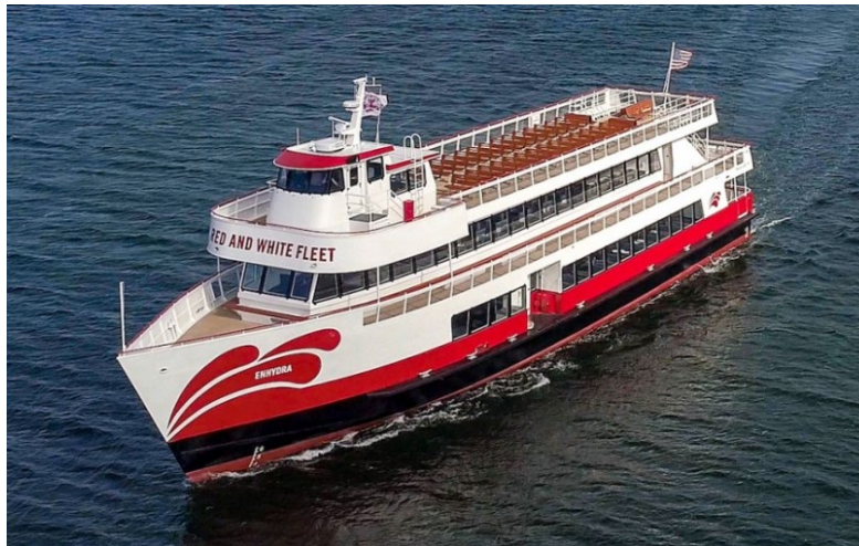
Figure A-16. Red and White Fleet’s Battery Plug-in/Diesel-Electric Bay Area Excursion Vessel, Enhydra
