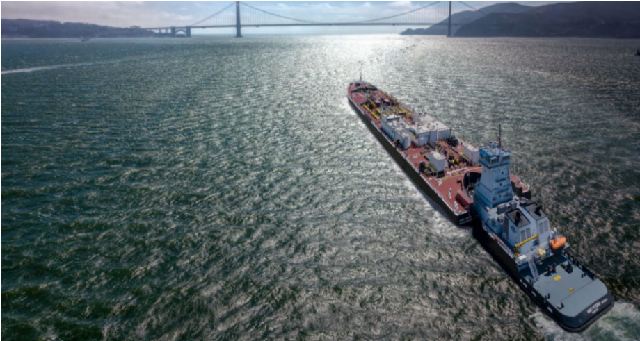
Figure A-2. Sause Bros. Ocean Double-Hull Fuel Barge, Alsea Bay
