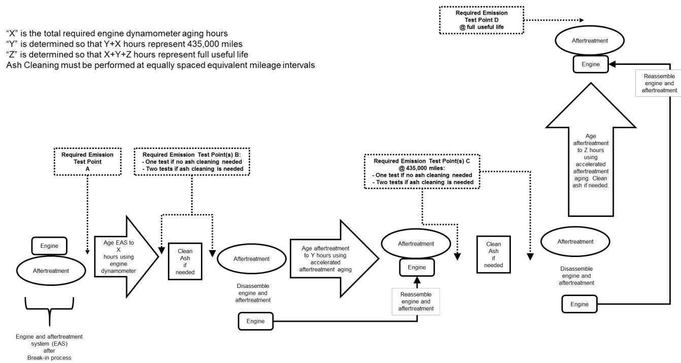
**Figure CA26-4: Alternative Durability Demonstration Using Accelerated Aftertreatment Aging for 2027 and Subsequent Model Year Heavy Duty Engines**
