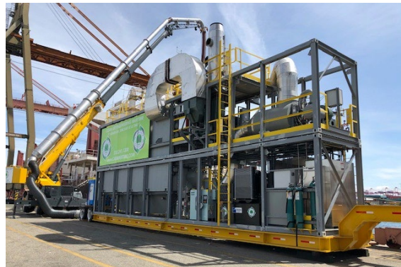
Figure ES-16: Land-based Capture and Control System
