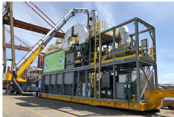
Figure I-23: Land-Based Capture and Control System
