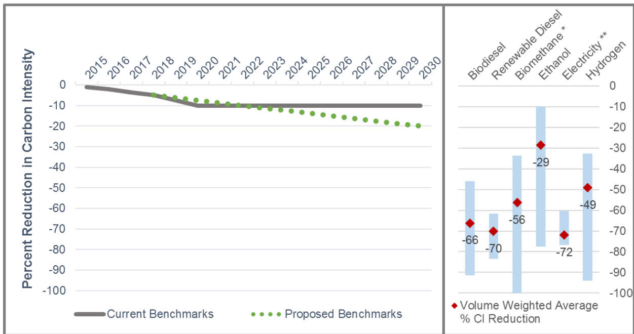
Figure EX-1: Current and Proposed Annual Carbon Intensity Benchmarks as Compared to CI Reductions Achieved in 2017 by the Most Common Alternative Fuels
