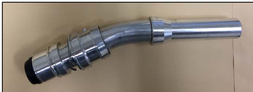
Figure 7: Previously Certified Assist Nozzle Spout Assembly (Prone to Loose Latching)
