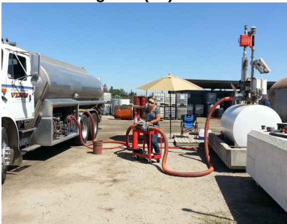
Fuel Transfer from Cargo Tank to AST
