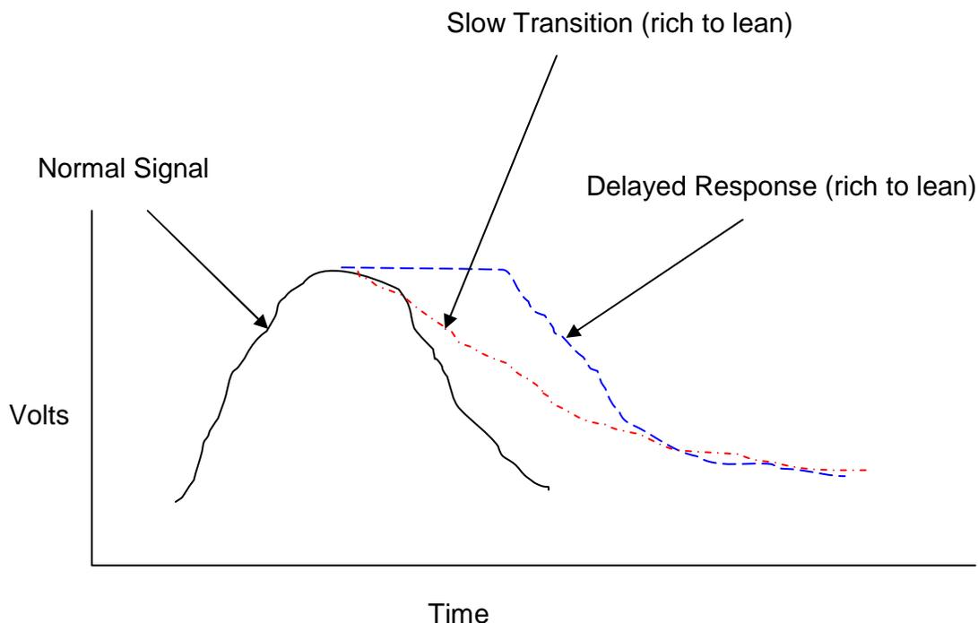
Results from testing in-use light- and medium-duty gasoline vehicles by ARB staff have also reinforced the need for more rigorous monitoring of the secondary sensors used to monitor the catalyst for proper operation. For secondary oxygen sensors, the HD OBD
