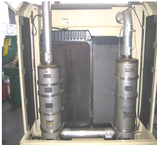
Figure VIII-3 - Photo of a Combination DPF and SCR System
