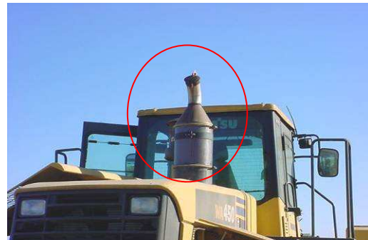
Figure VIII-2 - Photos of DPF Installations on Construction Vehicles
