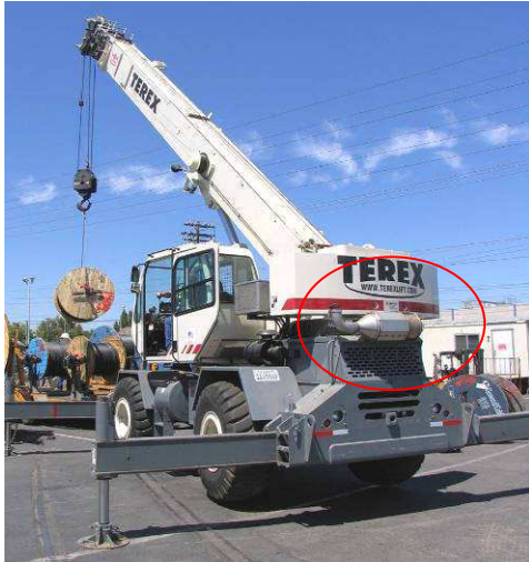
Figure VIII-2 - Photos of DPF Installations on Construction Vehicles
