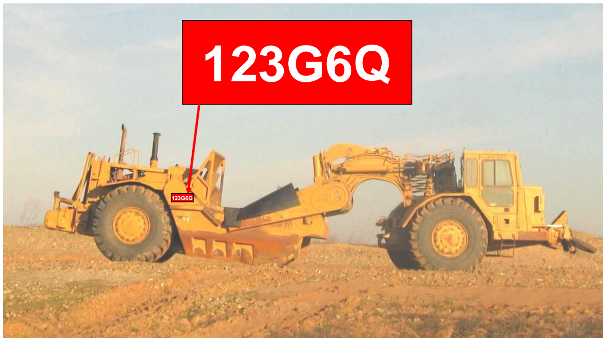
Figure VII-6 - Mock-up of how Equipment Identification Number Would Appear on a Scraper
