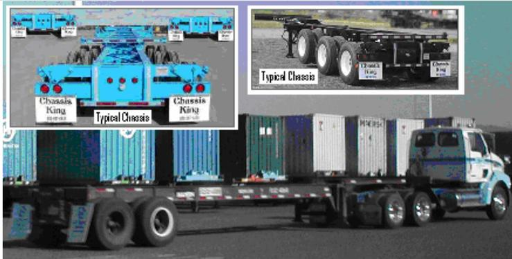
**Container Trucks – tractor with a container loaded on a flat bed chassis trailer (the container length is typically 20' or 40'). Note Port Container trucks will be carrying a container with vertical ribs (see below).**
