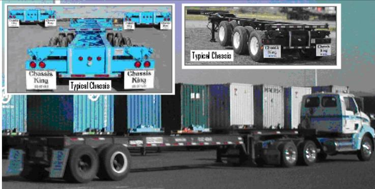
**\*Caution :** Container chasses are “I”-Beam chasses (as in above pictures). A flatbed chassis is not a container chassis and should not be counted as a chassis in our survey. An example of flatbed chassis is below:
