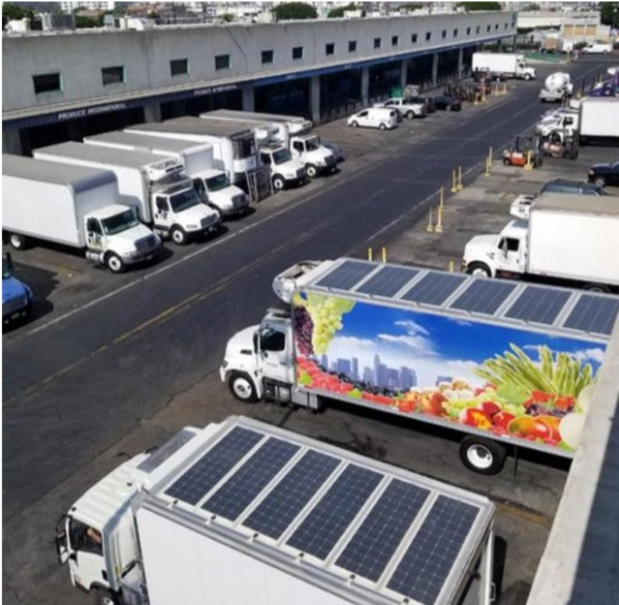
Figure IX-1. Battery-Electric Truck TRUs with Solar Assist
