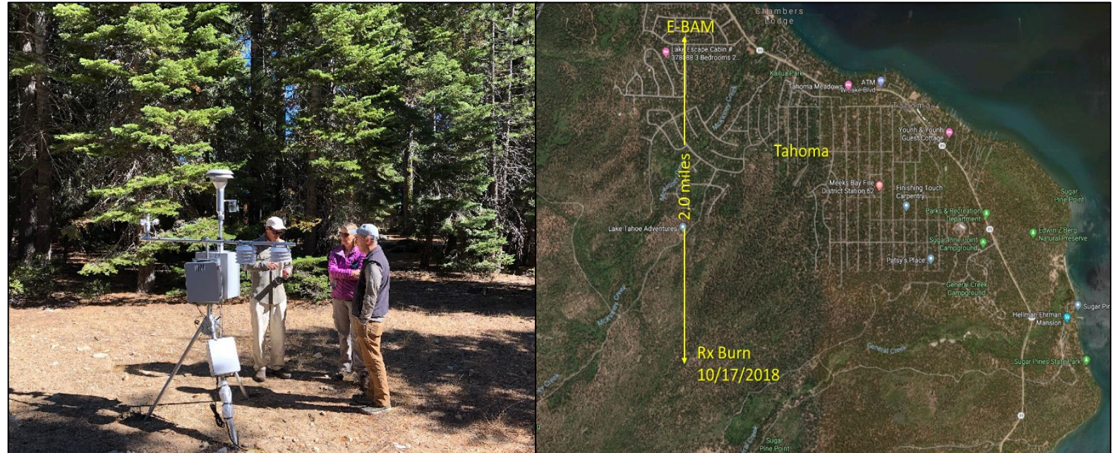
Environmental Beta-Attenuation Mass Monitor (E-BAM) unit deployed to monitor a prescribed fire at Sugar Pine Point State Park, October 2018
