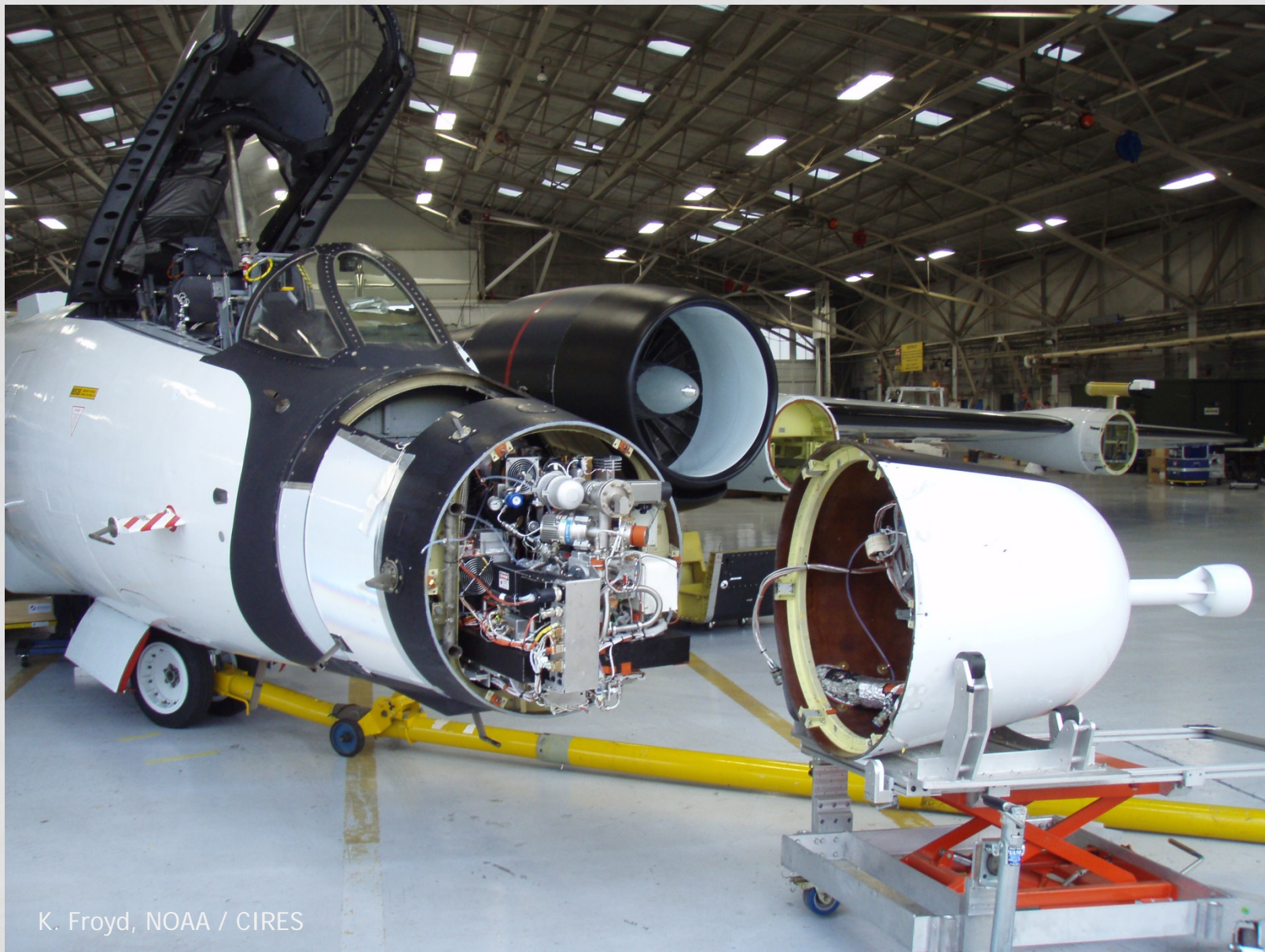
NOAA'S PARTICLE ANALYSIS BY LASER MASS SPECTROMETRY INSTRUMENT ABOARD THE NASA WB-57 HIGH-ALTITUDE RESEARCH AIRCRAFT.
