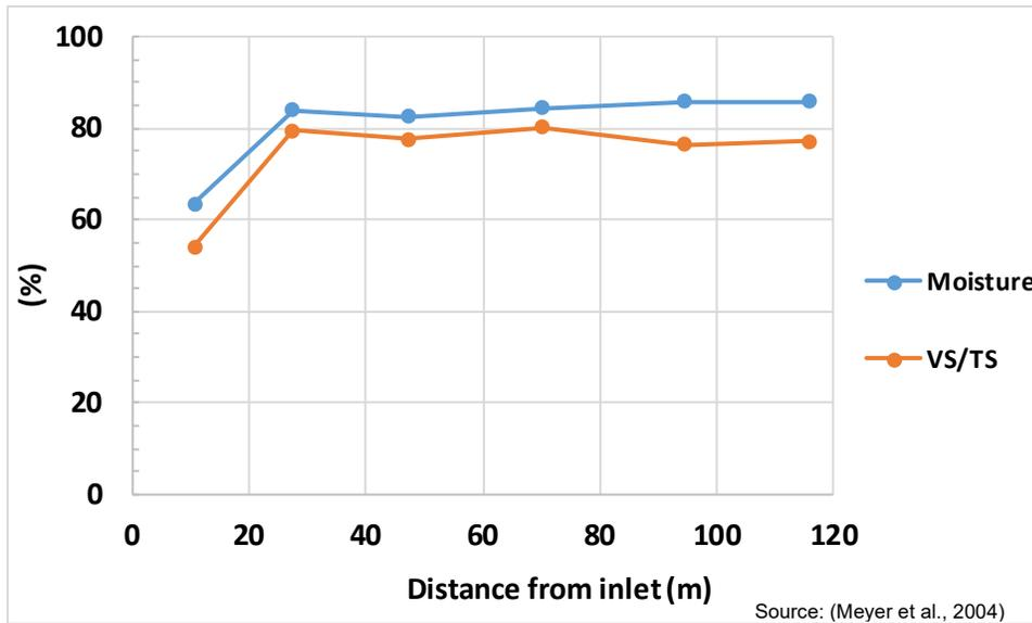
Figure 3-3 Moisture and volatile solids/total solids versus distance from inlet in a dewatered weeping wall cell
