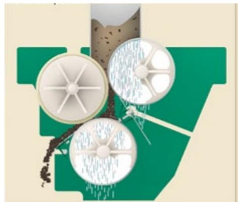
B. Cutaway of roller press
