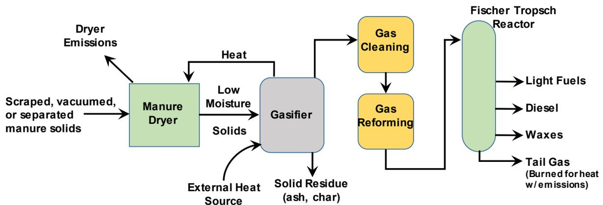
Figure 5-3 Schematic of the AWS manure-to-renewable diesel process.
