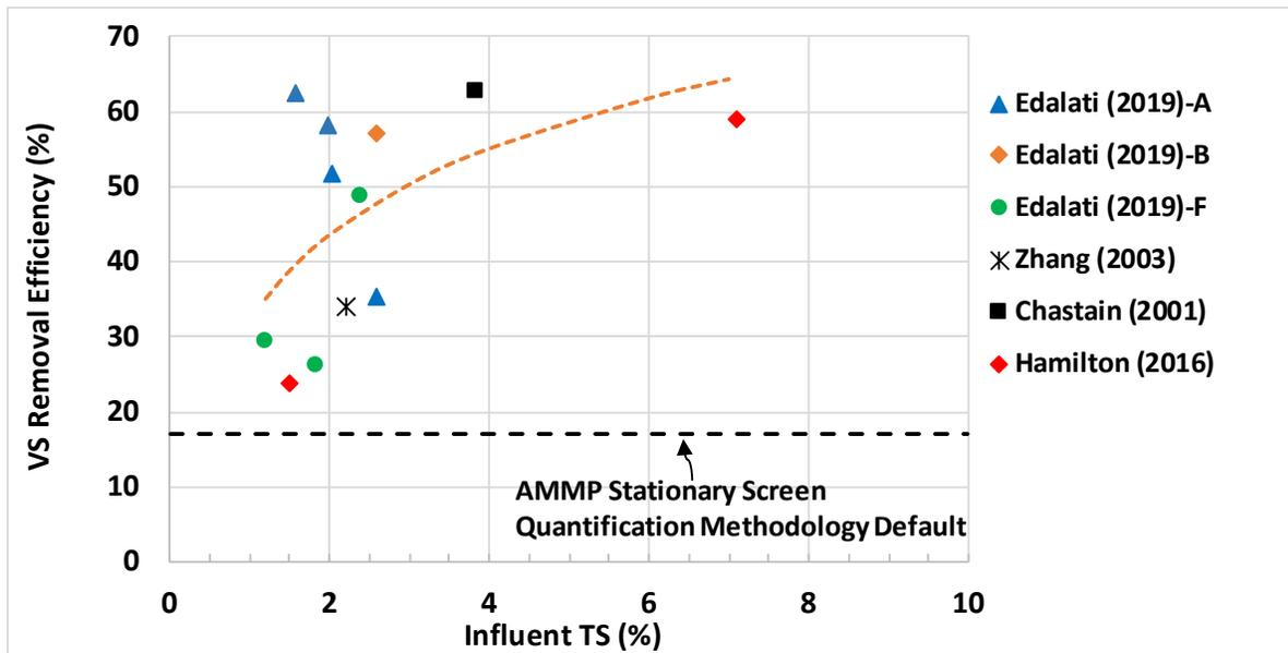
Figure 2-14. Volatile solids removal versus influent total solids concentration, sloped screen separators.
