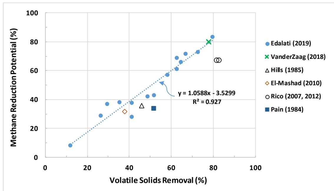
Figure 2-9. Methane reduction potential vs. volatile solids removal fraction from literature.
