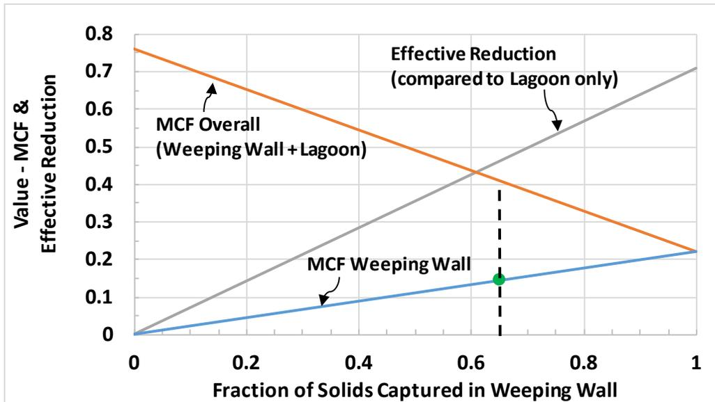
Figure 3-5 Effective weeping wall and overall methane conversion factors versus fraction of solids captured.
