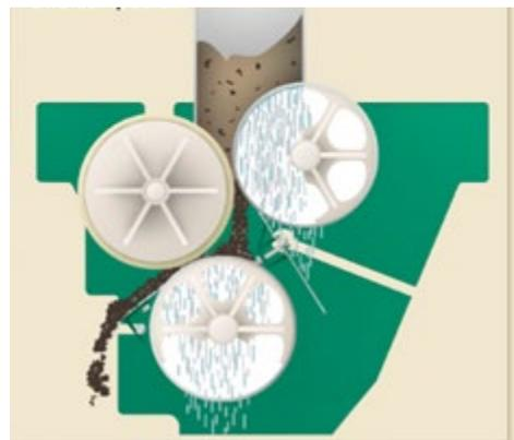
B. Cutaway of roller press
