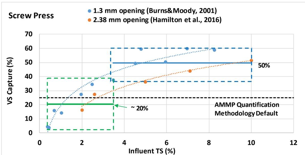
Figure 2-18. Screw press efficiencies; flush and slurry manure.
