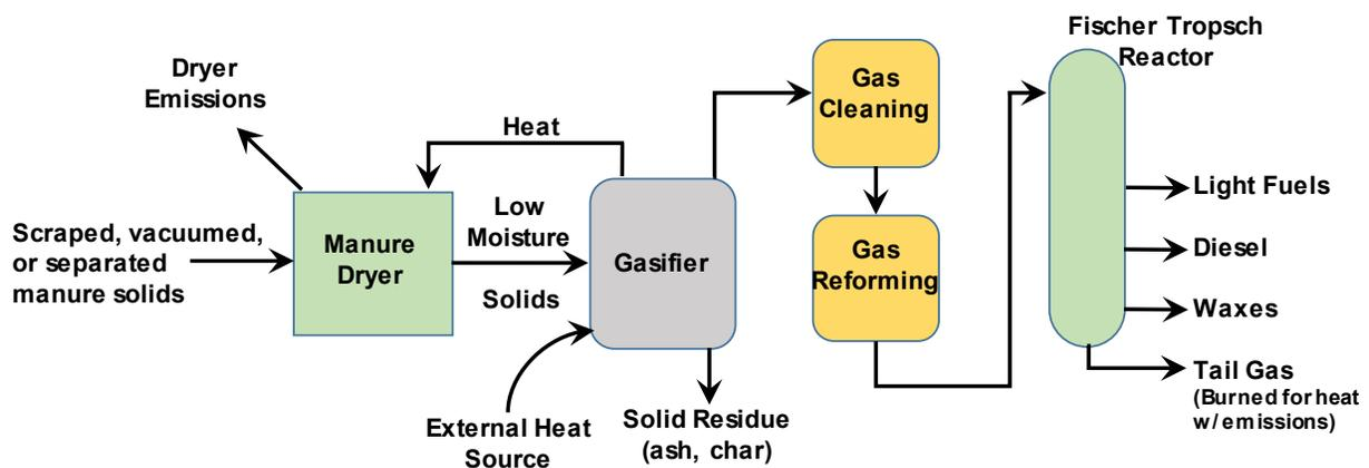
Figure 5-3 Schematic of the AWS manure-to-renewable diesel process.
