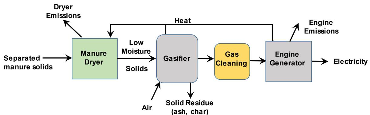
Figure 5-4 Schematic of a manure gasifier-to-engine generator system.
