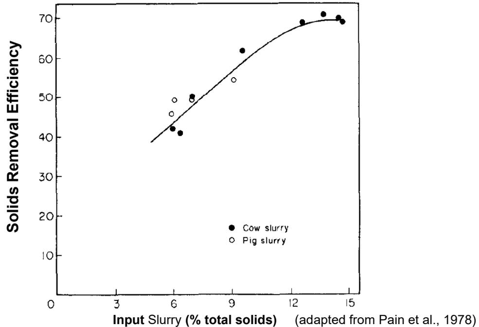
Figure 2-13 Relationship between input total solids and solids removal efficiency for a rotary screen separator
