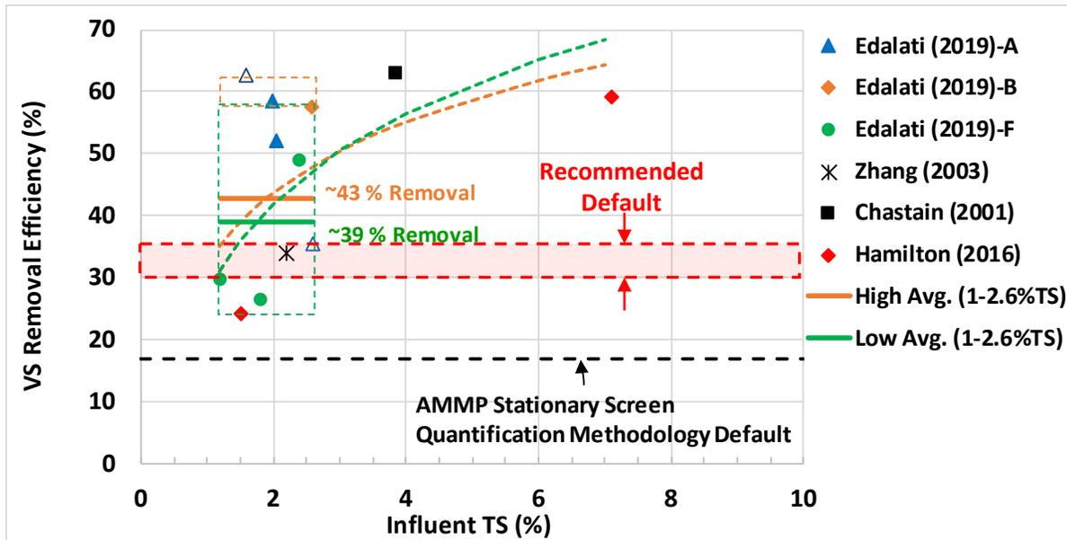
Figure 2-16. Recommended Quantification Methodology default for sloped screen separators
