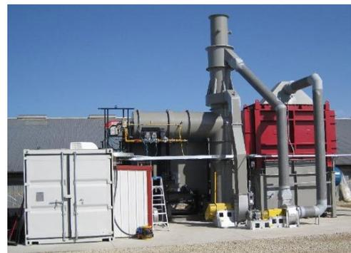
Figure 5-2 Schematic and photo of the Coaltec gasifier-close-coupled-combustion system.
