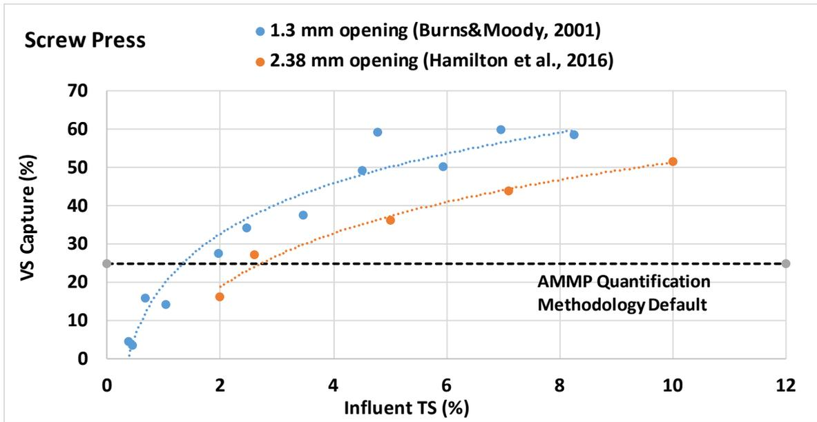
Figure 2-17. Volatile Solids removal versus Influent Total Solids Concentration; screw press.
