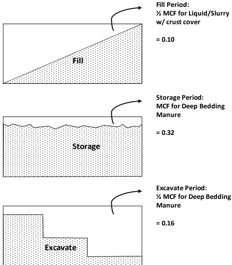
Figure 3-4. Representation of effective methane conversion factor fill, storage, and excavate phases of the weeping wall cycle
