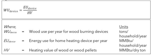
**Equation 9**. The annual wood use for wood burning devices is calculated as the Energy use for home heating device per year from Equation 3 multiplied by the heating value of wood or wood pellets.
