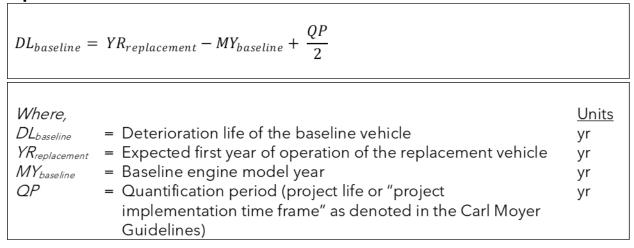
Equation 11 is used to determine the deterioration life in the replacement scenario if the replacement truck is brand new.
