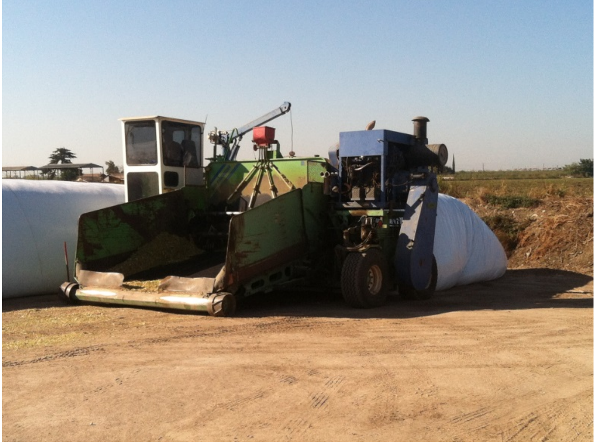
Photo 2. The open tray area for chopped corn collection, and the silage bags (white) being filled at the dairy.
