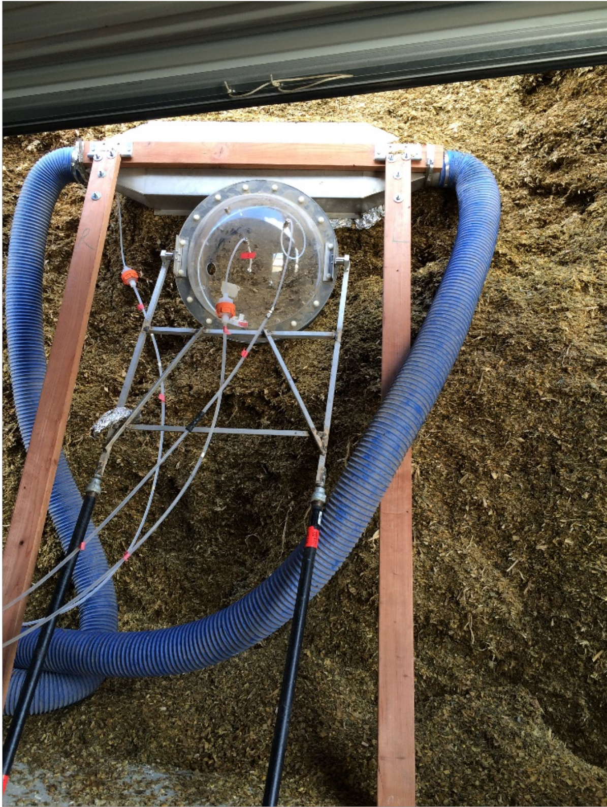
Photo 3. Flux chamber and wind tunnel sampling silage face within protective shipping container.
