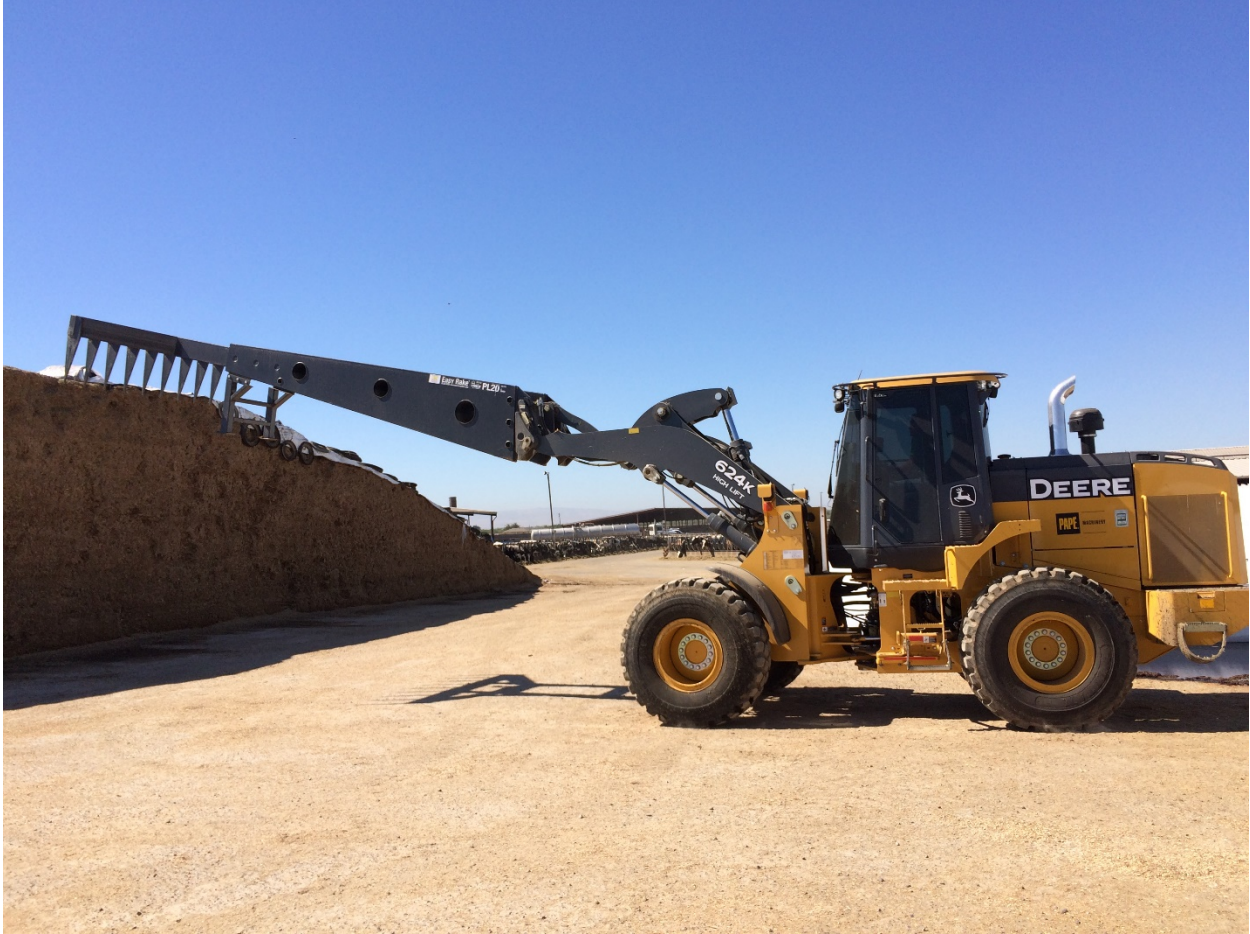
Photo 5. Standard front-end loader with quick connect to EZ rake attachment.
