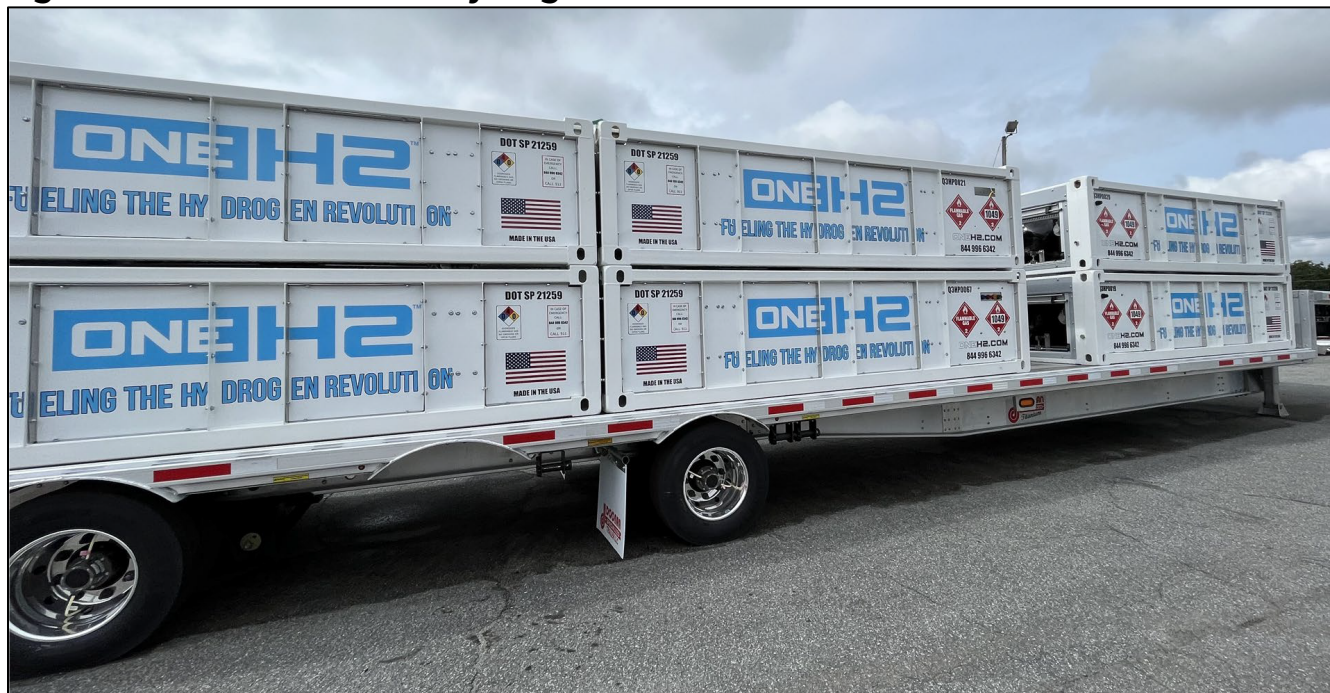
Figure 58: One H2's Mobile Hydrogen Refueler 281
