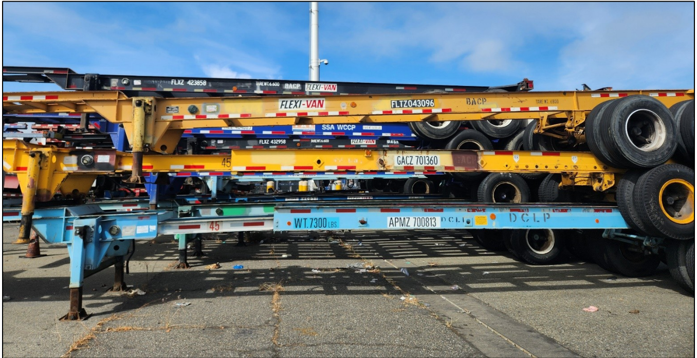
Figure 13: Stacked and Flipped Container Chassis (Staff photo)
