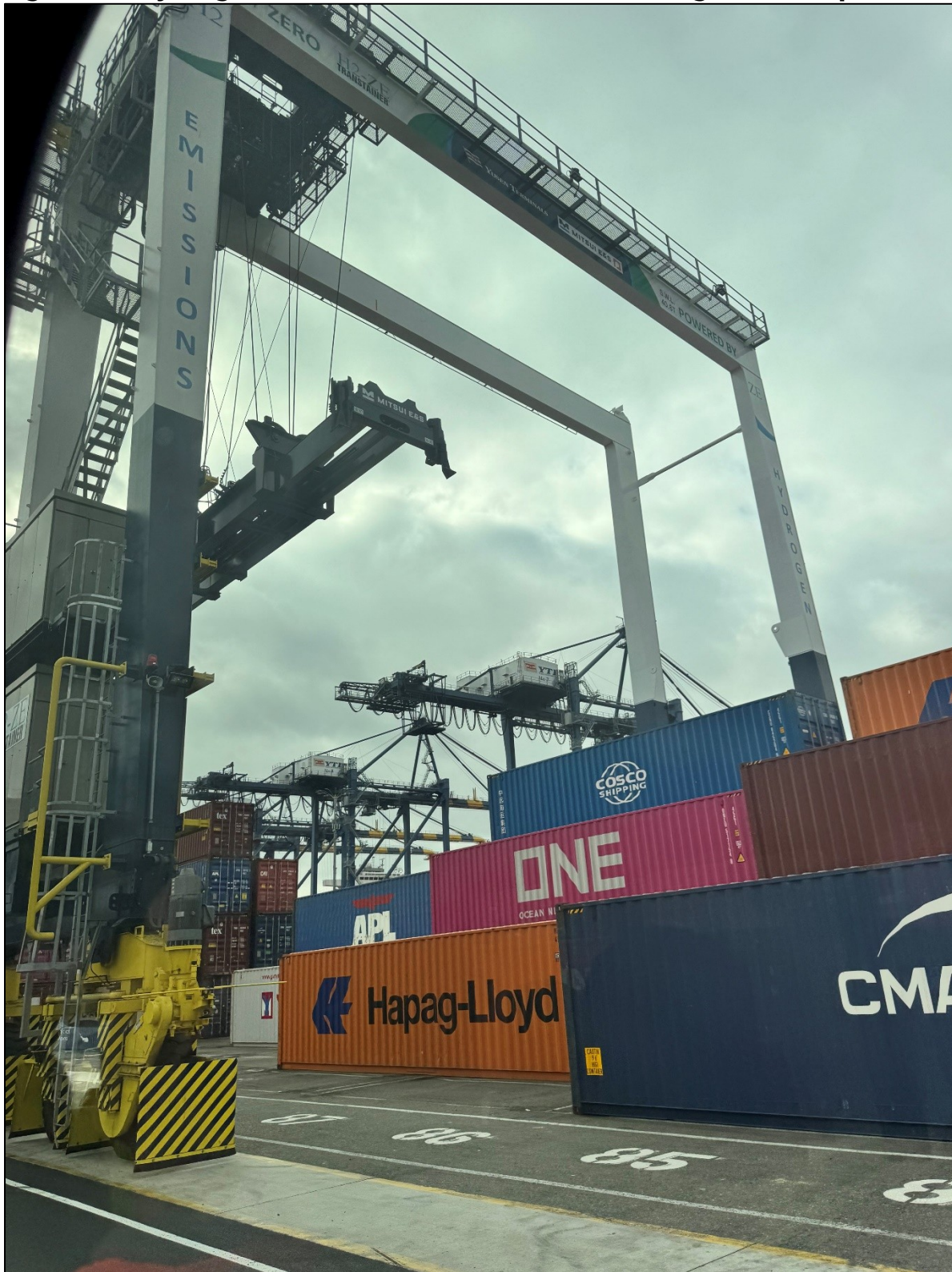
Figure 54: Hydrogen Fuel Cell RTG at the Port of Los Angeles (Staff photo)
