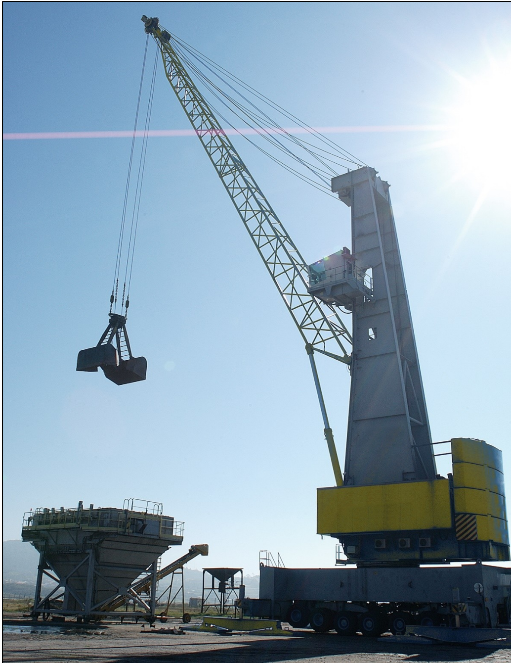
Figure 3: Mobile Harbor Crane with Grab Bucket
