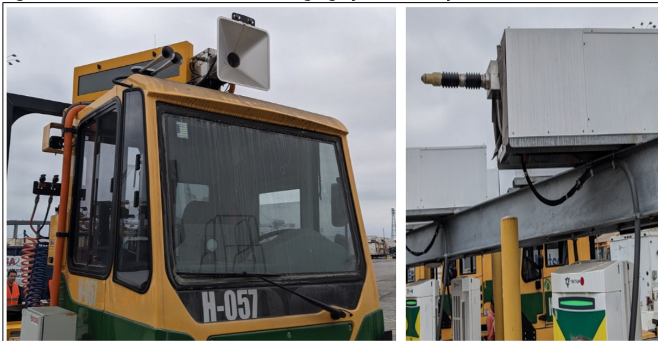
Figure 45: Hands-Free Conductive Charging System (Staff photo)
