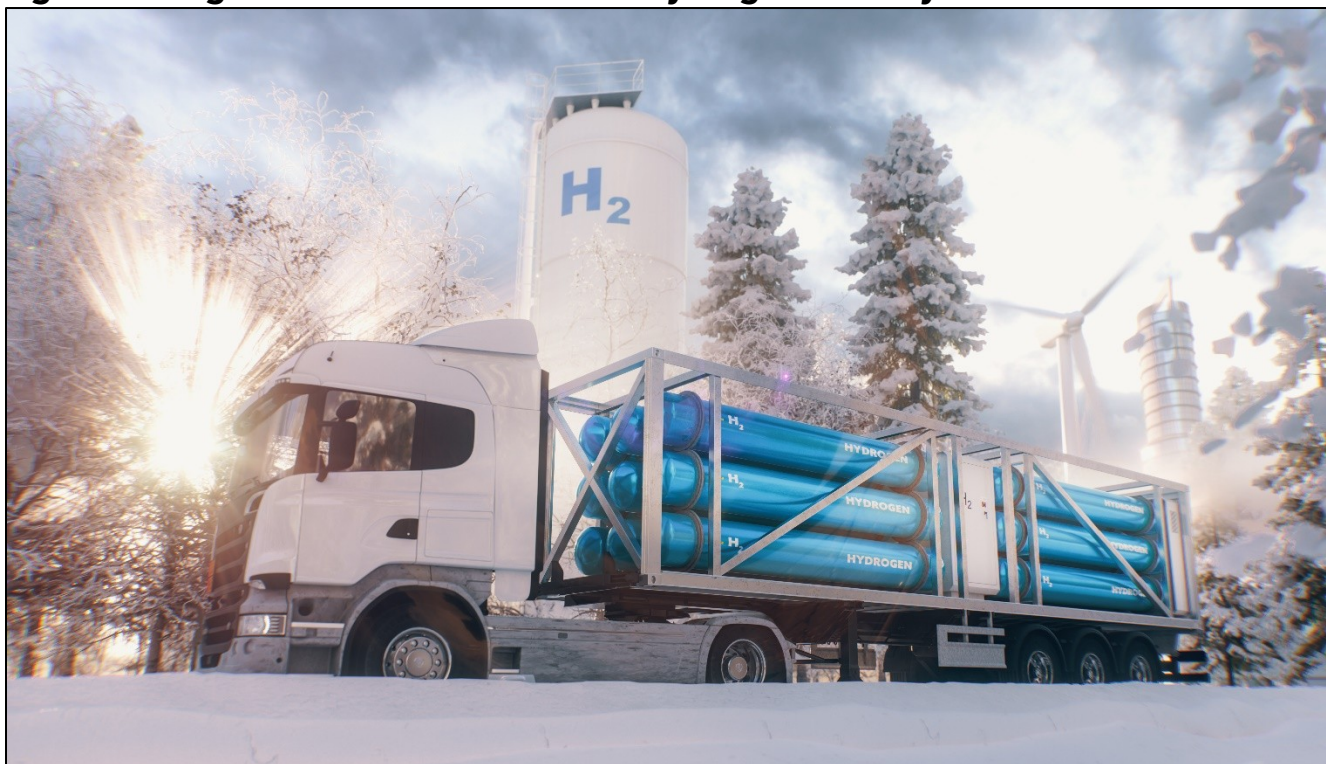
Figure 56: High Pressure Tube Trailer for Hydrogen Delivery
