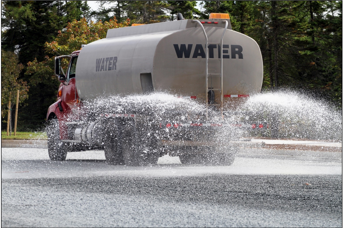
Figure 34: Cab-and-Chassis Truck Fitted with Water Tank, Nozzles, and Connectors
