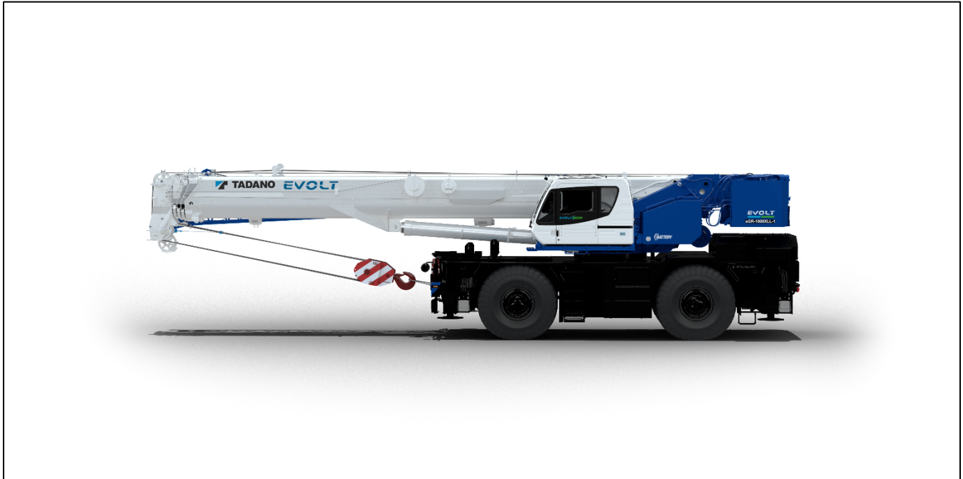
Figure 5: Battery-Electric Off-Road Wheeled Crane (Tadano)
