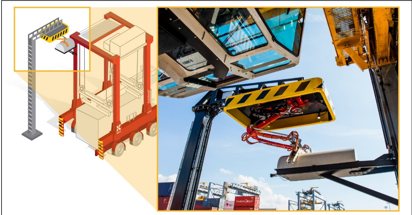
Figure 39: Pantograph Charging System for Battery-Electric Straddle and Shuttle Carriers (Kalmar)
