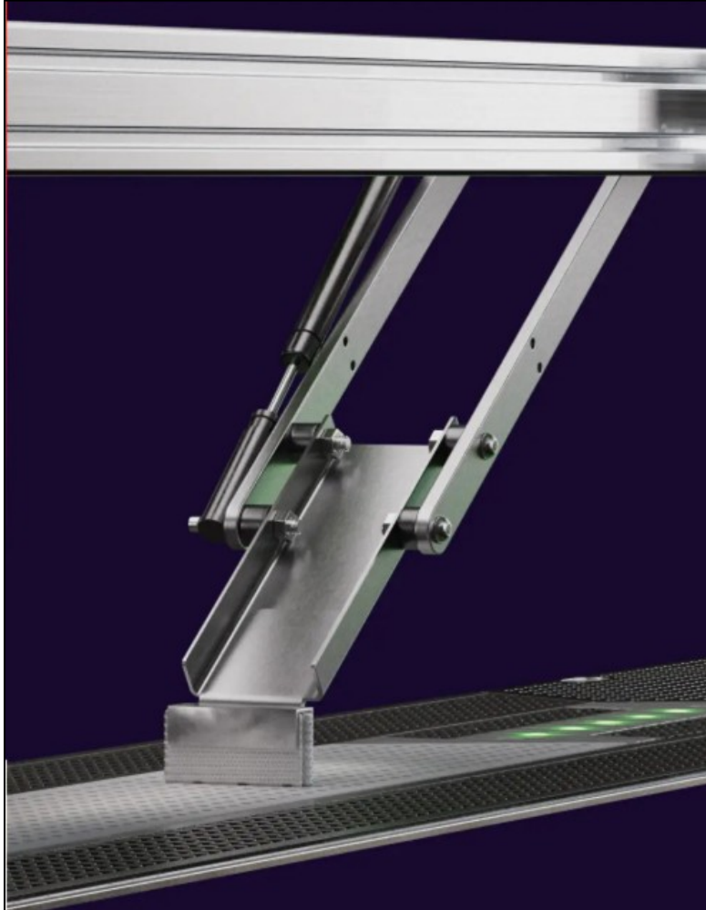
Figure 49: Retracting Conductive Arm (Elonroad)
