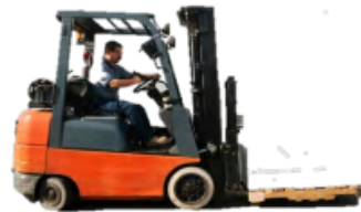
Class IV Internal Combustion Indoors, Smooth Floors & Loading Docks
