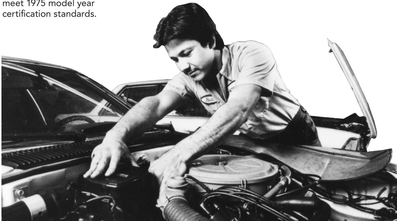
A certified mechanic inspects the car's emission control system, as part of the California Smog Check Program. July 1984.
