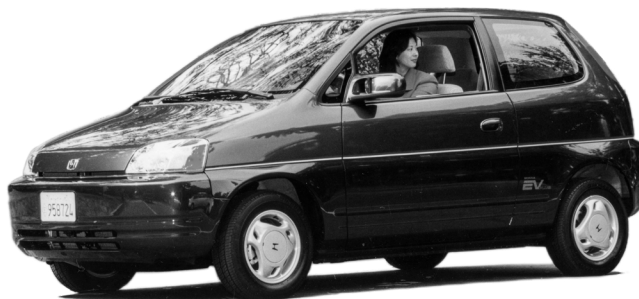
The Honda EV Plus, the first battery-electric vehicle from a major automaker with non-lead acid batteries.
