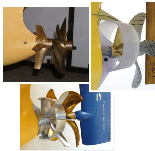
Figure 16. Examples of advanced propellor designs for OGV from Reference [209].
