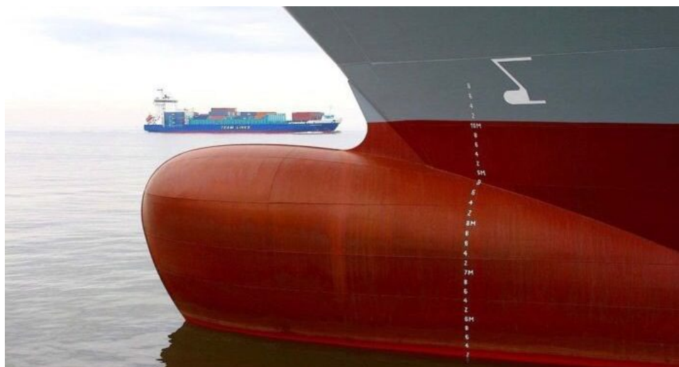
Figure 15. A bulbous bow typical of OGV from Reference [211]
