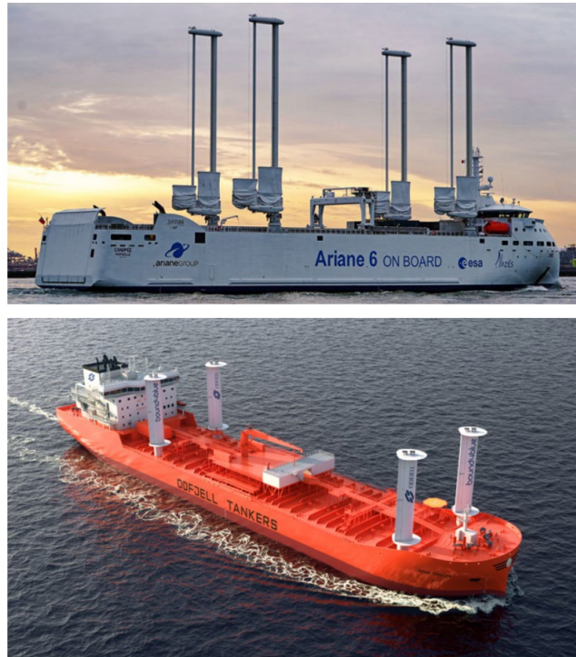
Figure 17. Two examples of wind assist technologies for OGV from Reference [209].
