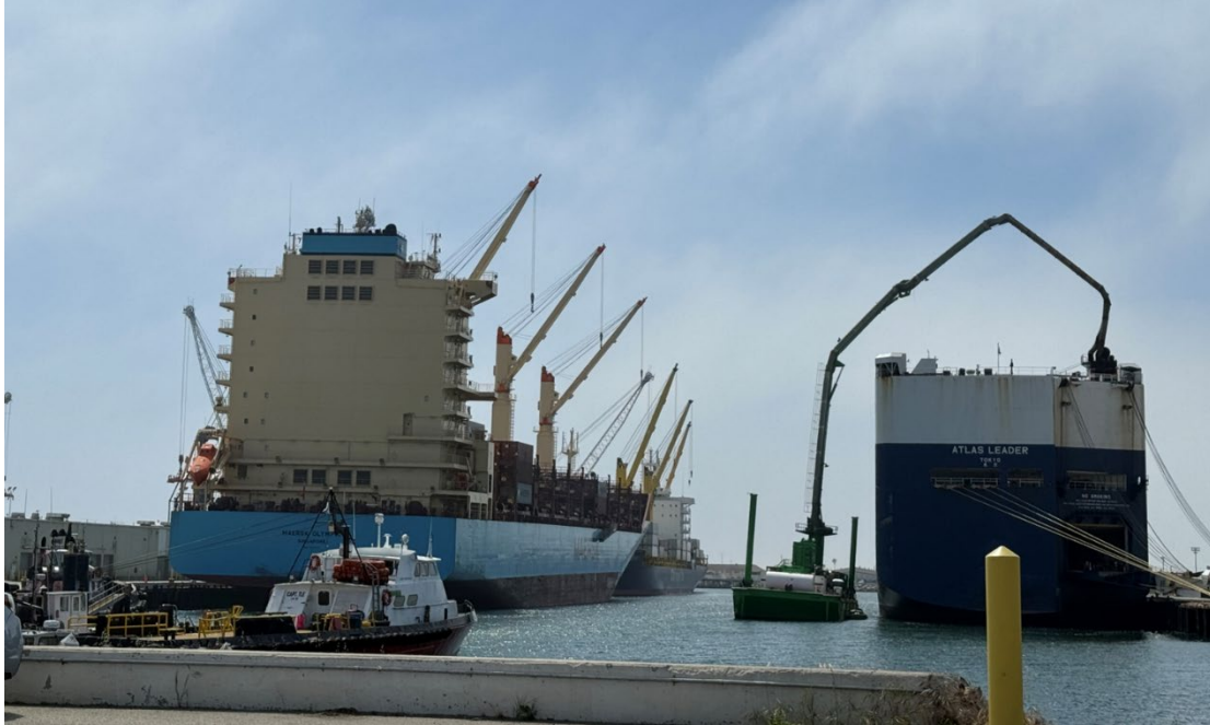
Picture 1. ECCS Barge Servicing RORO vessel
