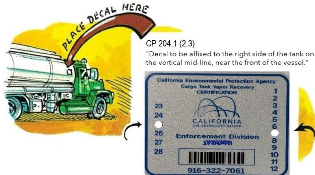
2. **Cargo Tank Number.** The CARB-issued Cargo Tank Number for the vessel should be displayed on the cargo tank in a location that can be visible. (CP 204.1 (2.3)). The preferred location is on the left side of the tank, either stamped on the first tank mount or as a vinyl numerical decal on the vertical mid-line near the front.
