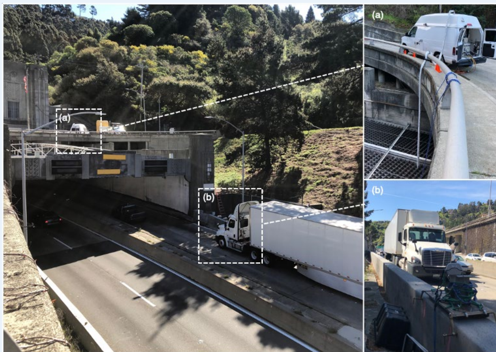
Figure 1. A van using monitoring equipment on an overpass at the Caldecott Tunnel Caltrans facility. Exhaust from a heavy-duty truck is sampled as it travels eastbound on Highway 24 and enters the tunnel. (a) The Van; (b) the roadside camera placed at the entrance to the tunnel.
