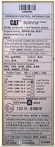
THIS ENGINE COMPLIES WITH U.S. EPA NONROAD AND STATIONARY AND CALIFORNIA OFF-ROAD REGULATIONS FOR 2022 DIESEL ENGINES ULTRA LOW SULFUR FUEL ONLY
