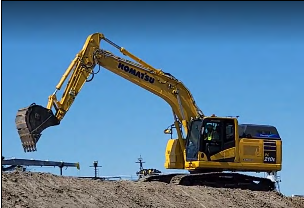
Figure 8: Battery-Electric Excavator (Staff photo)
