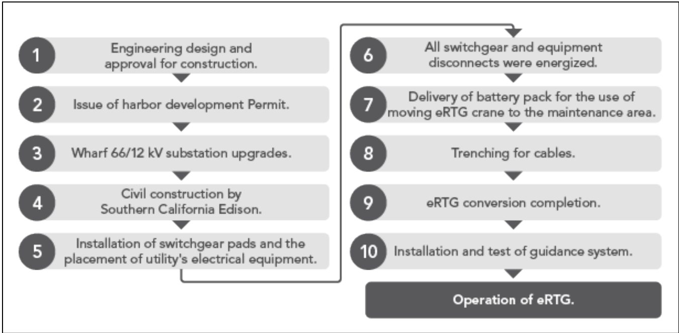
Figure 52: Diesel to Grid-Electric RTG Conversion Project Steps
