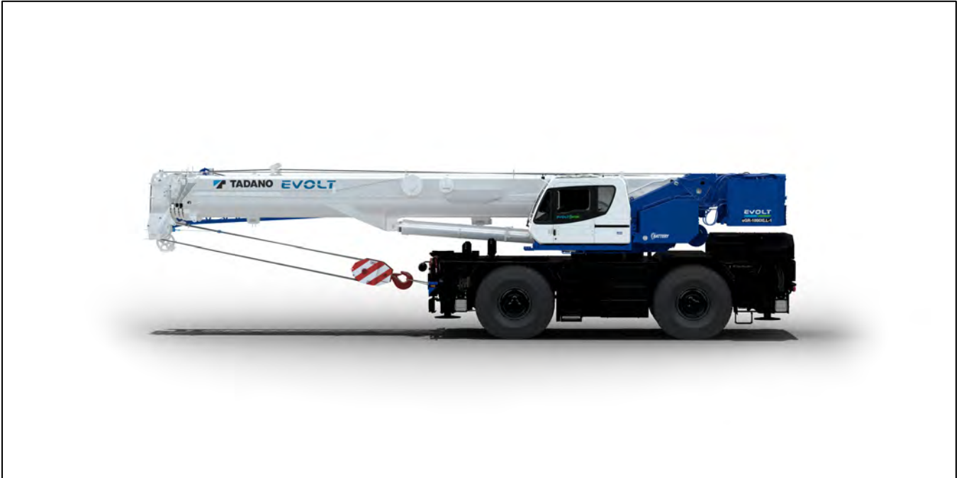
Figure 5: Battery-Electric Off-Road Wheeled Crane (Tadano)
