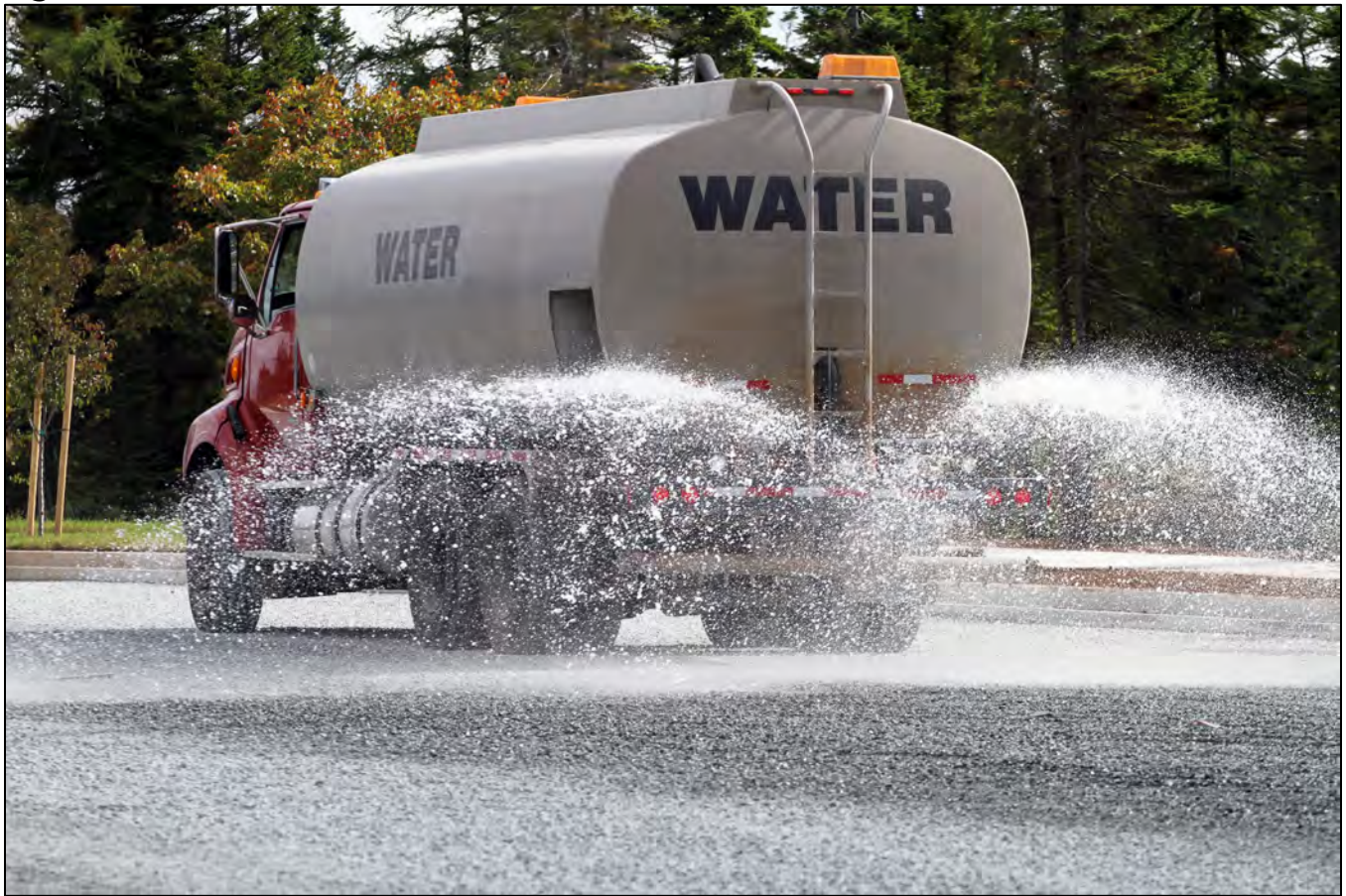
Figure 34: Chassis and Cab Fitted with Water Tank, Nozzles, and Connectors
