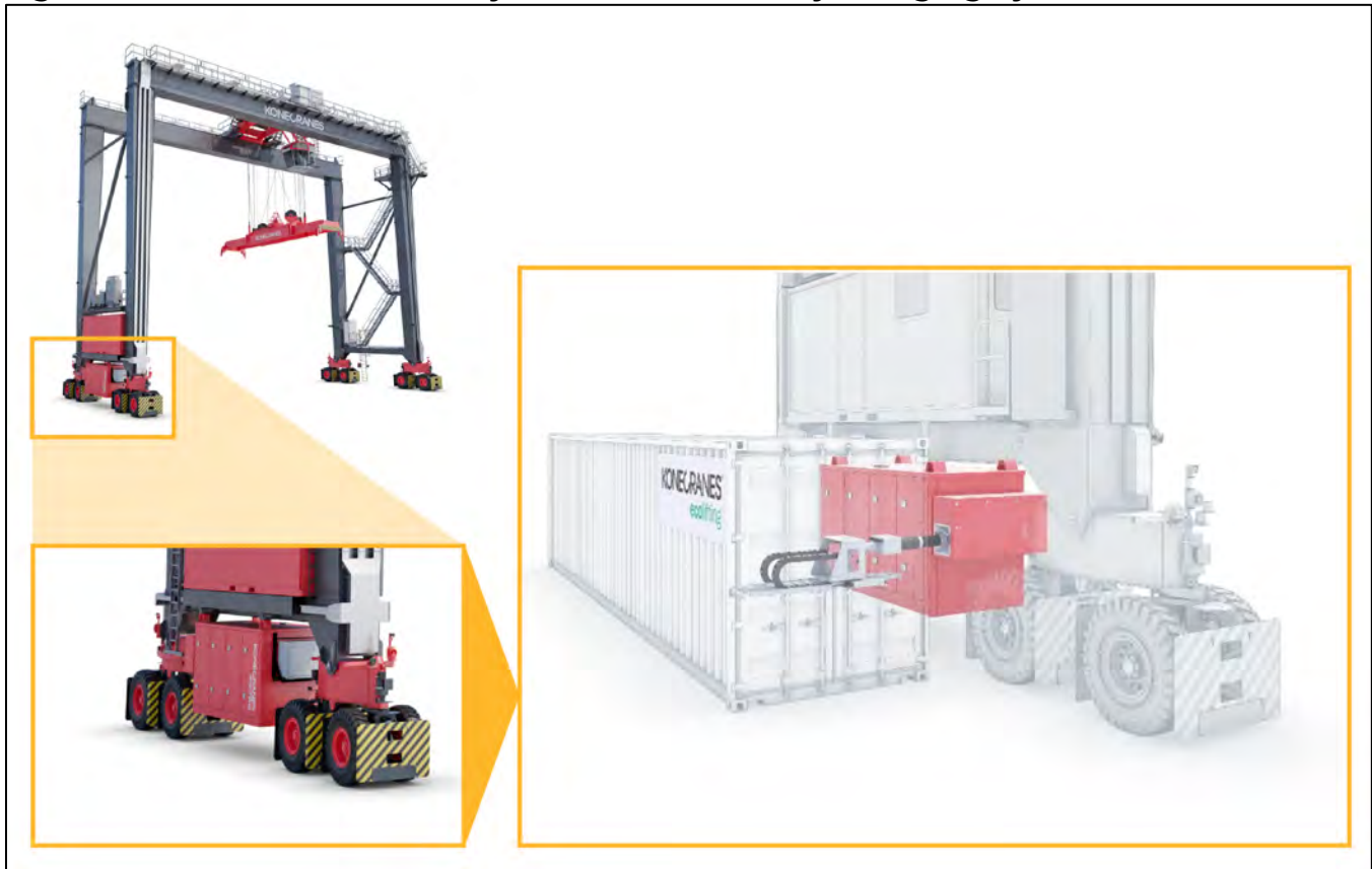
Figure 37: Illustration of Battery-Electric RTG Battery Charging System (Konecranes)
