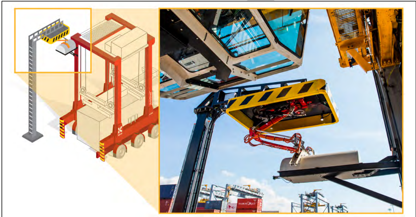
Figure 38: Pantograph Charging System for Battery-Electric Straddle and Shuttle Carriers (Kalmar)
