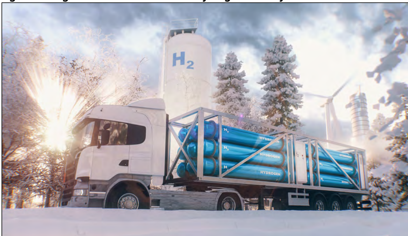
Figure 56: High Pressure Tube Trailer for Hydrogen Delivery
