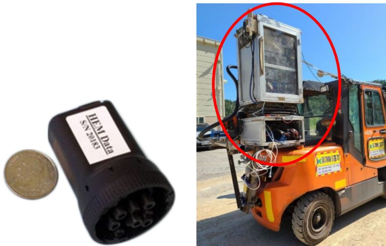
Figure 2 Photo examples of HEM data logger (left) and PEMS equipment (right)
