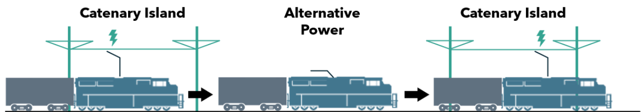
Figure 2: Discontinuous Overhead Catenary System Concept Diagram
