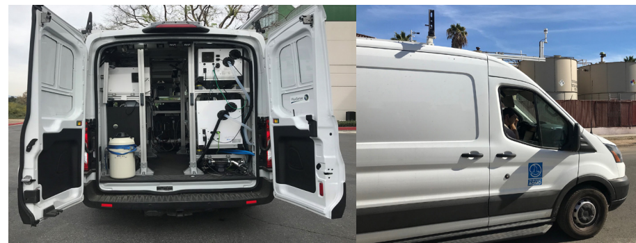
Figure 5. South Coast AQMD Optical Remote Sensing Mobile Laboratory (ORS-ML) conducting oil well site survey in WCWLB community (right); and of inside view of the air monitoring equipment aboard ORS-ML (left).
