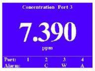
The 9000 Heated analyzer functions like the 9000 THA but is configured for single point analysis (with or without a sample pump) of samples heated up to 376 °F (191 °C) for pre-filtered (< 10 microns) noncondensing samples.
