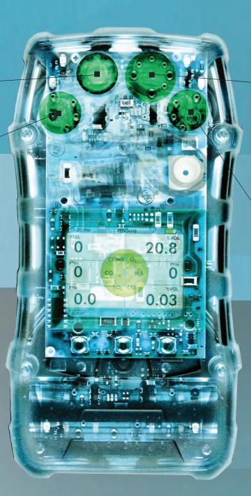
MSA XCell SO<sub>2</sub>, Cl<sub>2</sub>, or NH<sub>3</sub> Sensor
