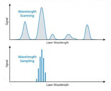
Figure 1. (top) True continuous wavelength scanning capabilities of OA-ICOS allow direct measurements of fully resolved absorption lineshapes. (bottom) Discrete wavelength sampling measurements recorded using CRDS do not provide detailed absorption lineshapes. As a result, OA-ICOS instruments report measurements with higher accuracy and linearity, and are much less susceptible to cross interferences and errors due to contaminants.
