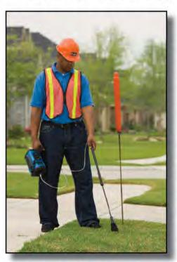
The **HEATH** Detecto Pak-Infrared (DP-IR") is a highly advanced technology capable of detecting methane without false alarming on other gases. The DP-IR is the latest generation of leak survey instruments from **HEATH** that will greatly improve the productivity and safety of a walking/mobile survey.
