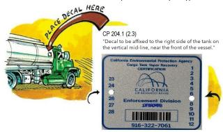
2. **Cargo Tank Number**. The CARB-issued Cargo Tank Number for the vessel should be displayed on the cargo tank in a location that can be visible. (CP 204.1 (2.3)). The preferred location is on the <u>left side of the tank</u>, either stamped on the first tank mount or as a vinyl numerical decal on the vertical mid-line near the front.
