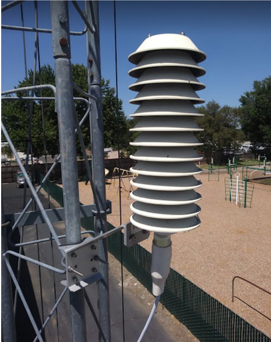
Figure 2: Field Installation of Vaisala in Solar Shield
