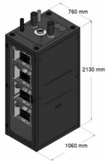
Hydrogen Fuel Cell Rack Dimensions
