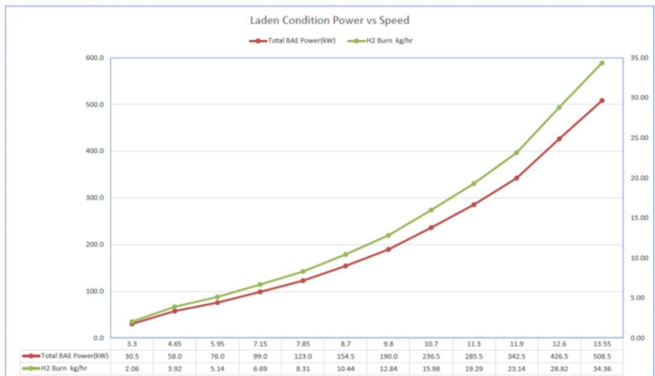
Figure #14 – Sea Change Speed vs. Power Curve
