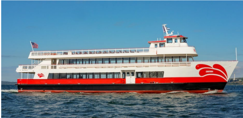
Figure 31: Plug-in hybrid diesel electric excursion vessel the Enhydra. From Reference [137].
