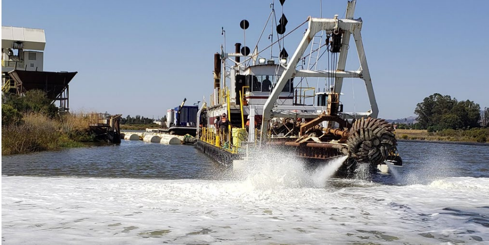
Figure 32: Sandpiper 18' Cutter Suction Dredge used to maintain Santa Barbara Harbor. Image taken from Reference [138].
