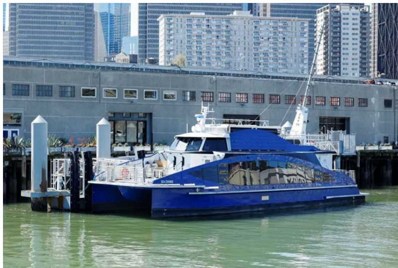
Figure 29: Sea Change fuel cell electric catamaran ferry. From Reference [129].
