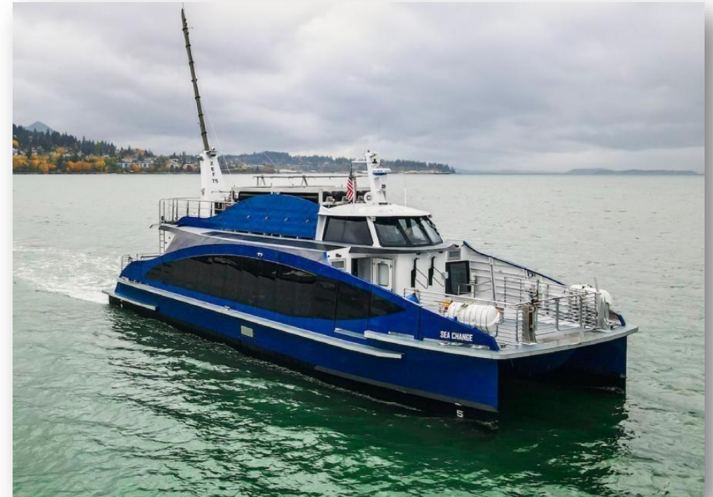
SEA CHANGE, hydrogen fuel cell passenger ferry. Source: SWITCH Maritime
