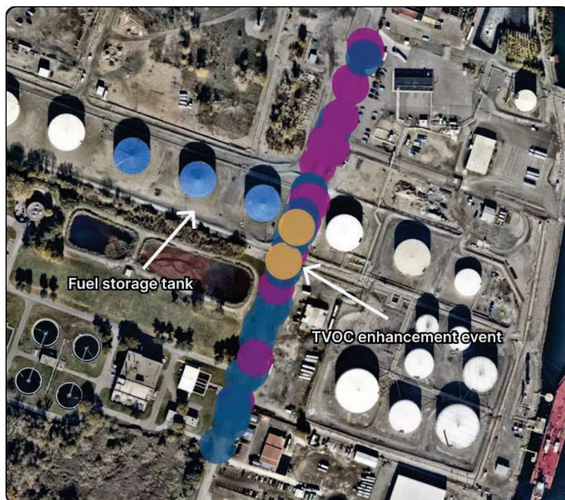
Figure 5.20: An example of a Level 3 analysis that displays TVOC enhancement events detected over a one year period in close proximity to fuel storage tanks, collected as part of larger monitoring effort over a wide area within this community. The individual events are classified according to other pollutants that are concurrently detected as enhancements, specifically combustion tracers (indicated in orange), indicating a likely combustion source, or other pollutants, for example methane (indicated as blue); TVOC detections in the absence of other pollutant enhancements are indicated in purple.
