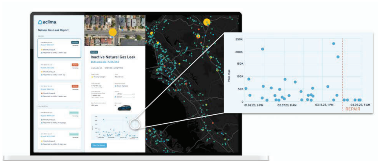
Figure 4.4: Example of an enhancement-based analysis of source identification of a natural gas leak
