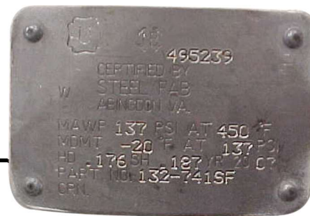
Clean Air Separator Data Plate
