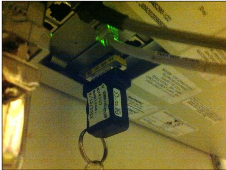
FIGURE 4 Maintenance Tracker Key Plugged Into TLS Console
