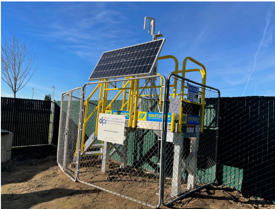
Figure 15: Air Sampling Equipment in Hughson, CA for Stanislaus County Seasonal Study
